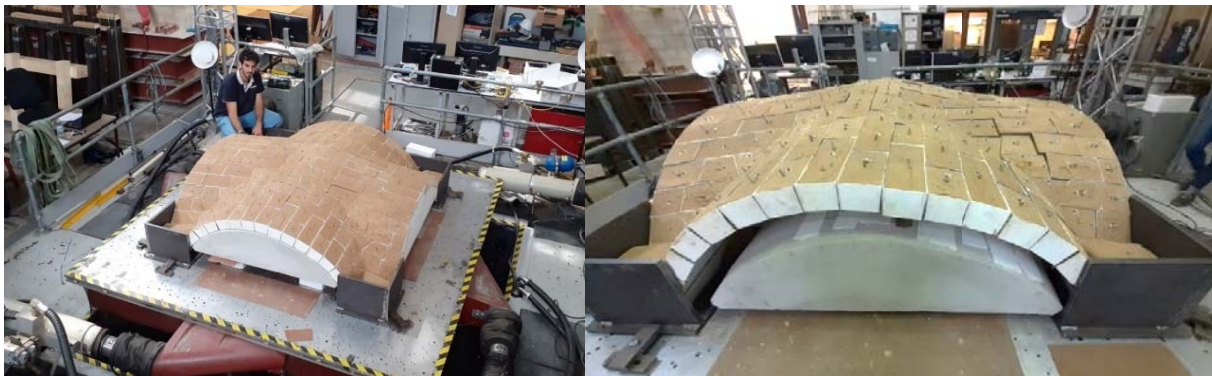
Fig. 14 - Physical model before the formwork removal and afterwards, showing the failure mechanism under gravity load.
