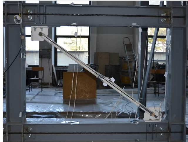
Fig. 9 – SHS brace and gusset plates
