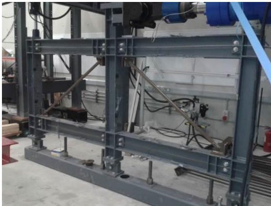
Fig. 3 – SC-CBF tested under cyclic static lateral loading (adapted from O'Reilly [14])
