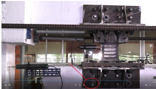
Fig. 9 – Unwittingly omitted important bolt not disposed in the tests
