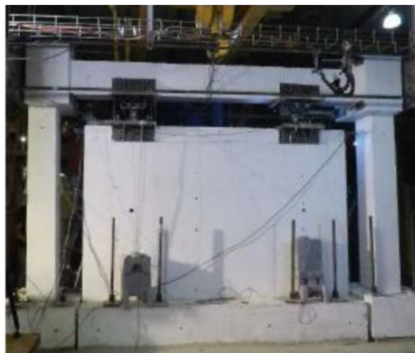
Fig. 4 – Reinforced concrete frame used in the test [3]
