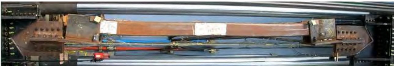
Fig. 8 – Global deformation of Specimen 5 at the first 2.5% EDR peak in tension
