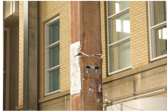
Fig. 6 – Low-cycle fatigue fracture in HSS of Specimen 5 (first 2.75% EDR cycle)
