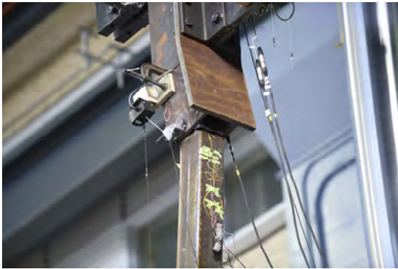
Fig. 5 – Fracture in HSS of Specimen 2 (first 2.0% EDR cycle)
