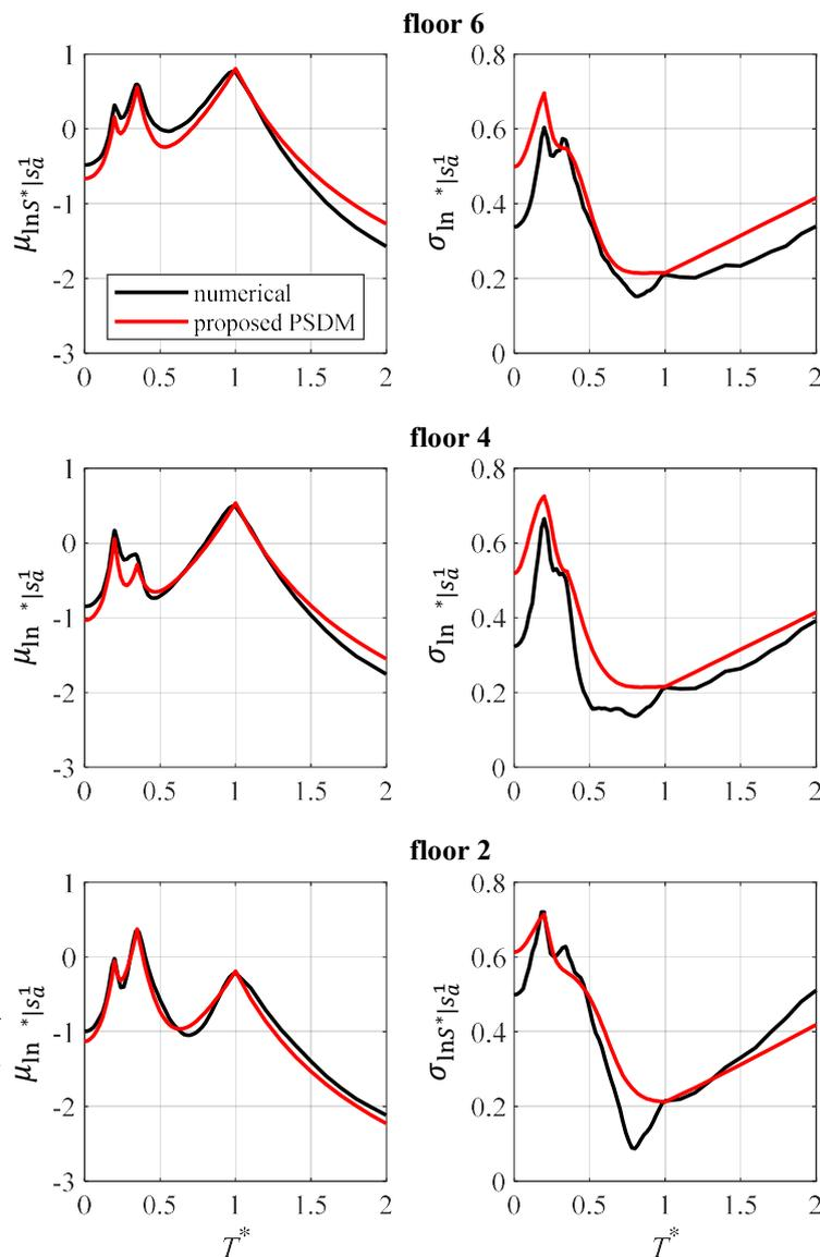
Fig. 5 – Parameters of the conditional PSDM of the floor spectral response obtained for the case study structure under a seismic excitation corresponding to a mean return period  $T_R = 500$  years
