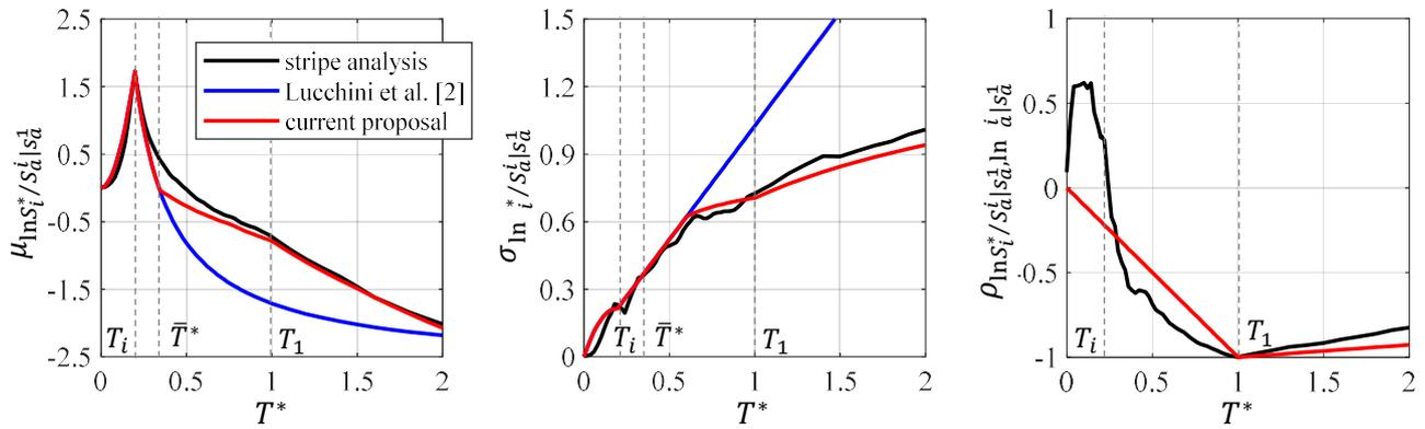
Fig. 2 – Prediction of the log amplification factor of the modal floor spectral response
