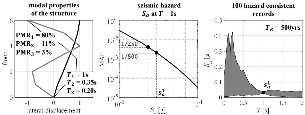
Fig. 4 – Case study structure: modal properties (left), seismic hazard at the site (center), and response spectra of hazard consistent ground motion records (right)
