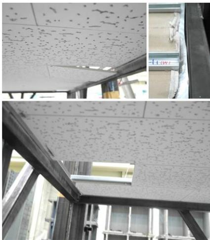
(a) Observed failure in IMC-L specimen (partial panel, molding, panel failure)
