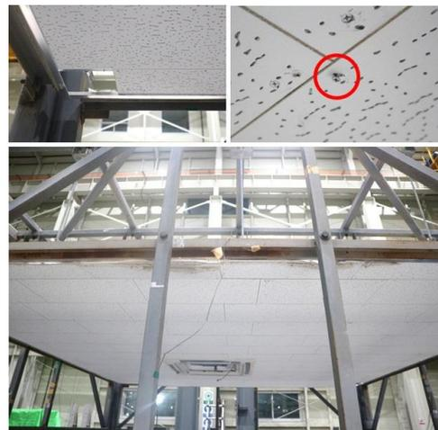
(b) Observed failure in IMC specimen (panel, screw, perimeter panel failure)
