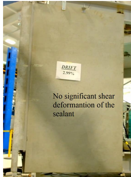
c. Front-view of inclined-corner sub-assembly
