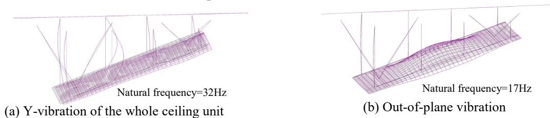
Fig. 12 – Natural frequency by FEM analysis
