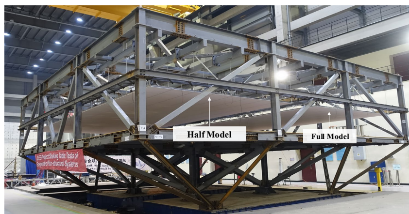
Photo 2 Overall view of the test specimen and supporting frame
