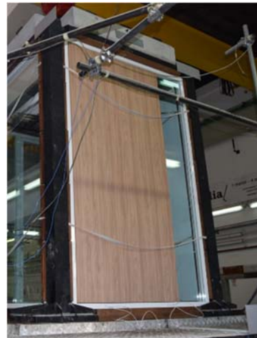
Fig. 3 - Mixed glass-wood partition
