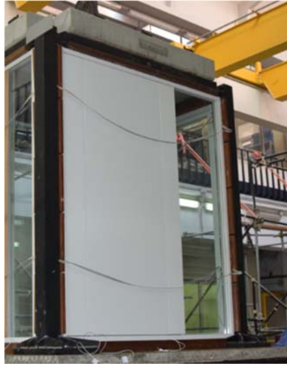
Fig. 4 - Mixed glass-steel partition
