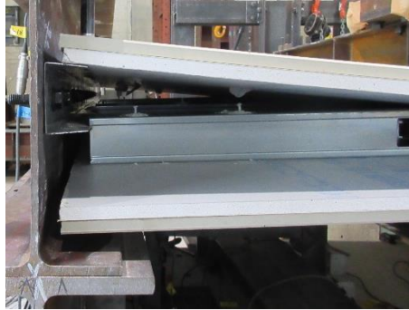
Fig.11 Slip-off of studs from the track of ceiling side
