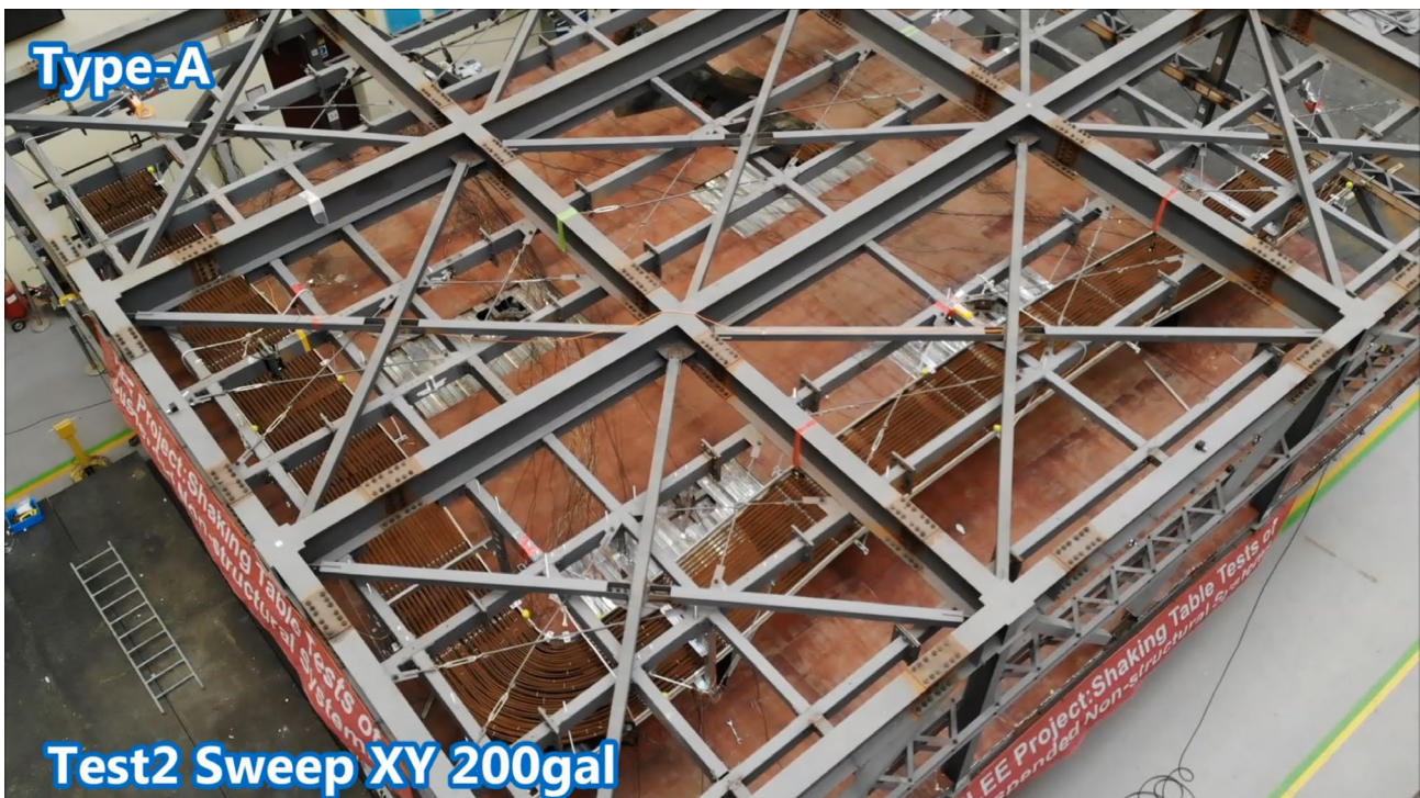
Photo 11 Cable Tray Test2 experiments taken with a drone
