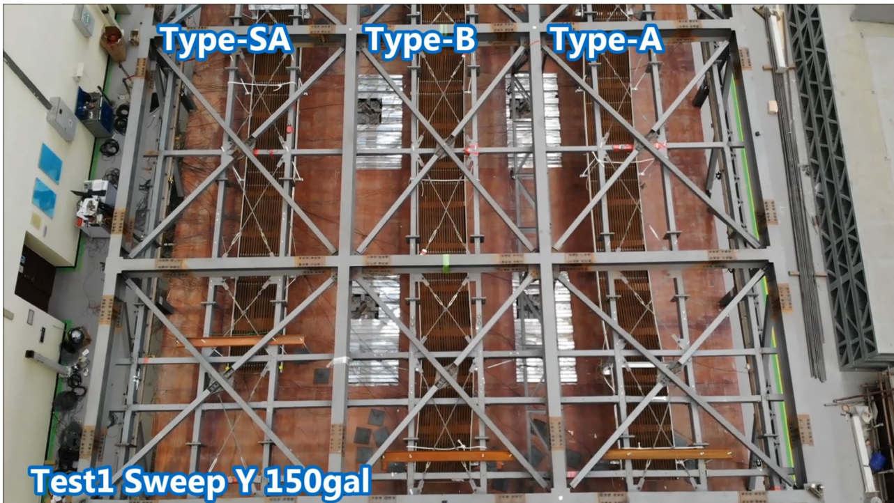
Photo 10 Cable Tray Test1 experiments taken with a drone
