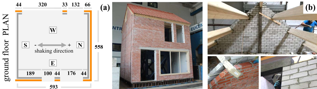
Fig. 2 (a) Ground floor plan (in cm), (b) EUC-BUILD6 and roof construction details [3]
