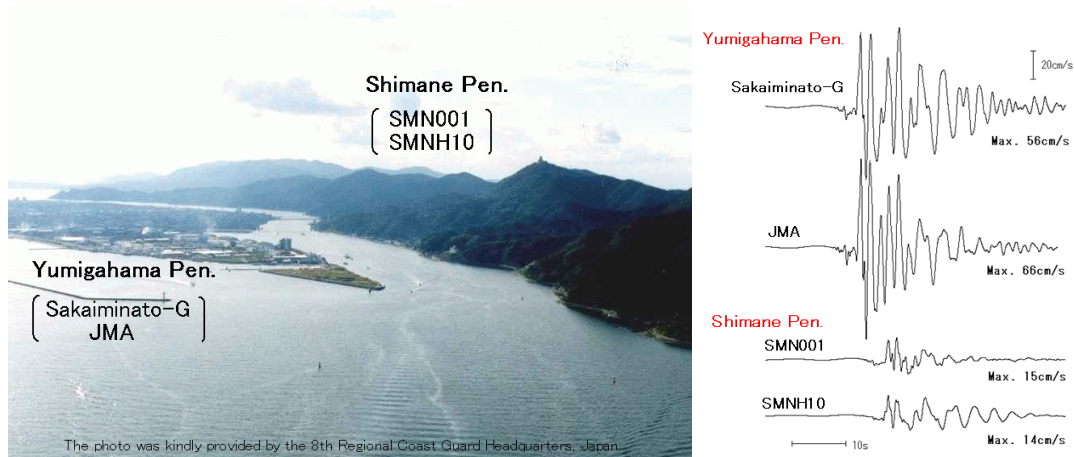
Fig. 5 – The topography around the Port of Sakai, west Japan (left) and the velocity waveforms for the fault-normal component recorded around the port during the 2000 Tottori-ken Seibu earthquake ( M_j 7.3 ).
