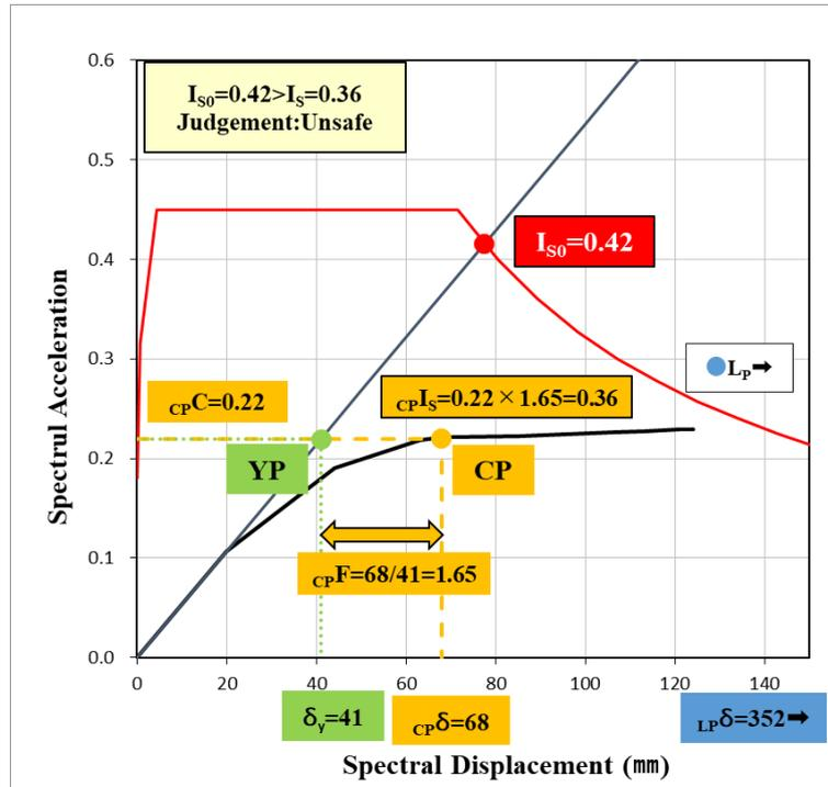
Fig. 12 –  $I_{S0}$  index and  $I_s$  index before retrofit
