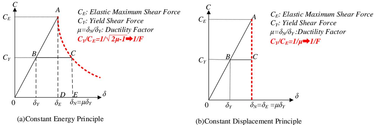
Fig. 1 – Constant Energy Principle and Constant Displacement Principle
