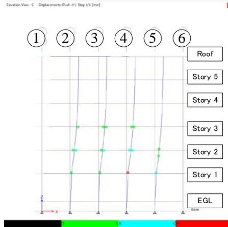
Fig. 15 – Plastic hinges at just first CP after retrofit (Grid C)
