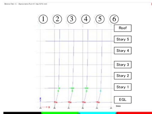
Fig. 11 – Plastic hinges at the final step (Grid C)
