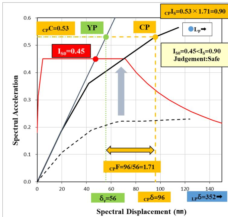
Fig. 16 –  $I_{S0}$  index and  $I_S$  index after retrofit
