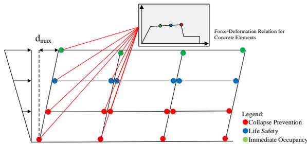
Fig. 2 –Example of hinge mechanism by pushover analysis
