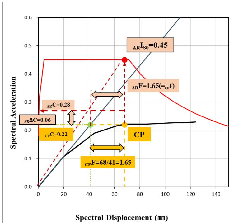
Fig. 13 – Example for estimation of required strength
