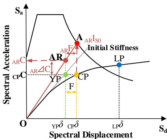
Fig. 7- Calculation procedure of the required strength at ground floor
