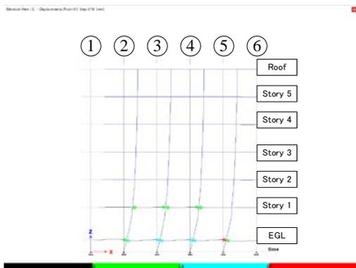
Fig. 10 – Plastic hinges at the first CP (Grid C)
