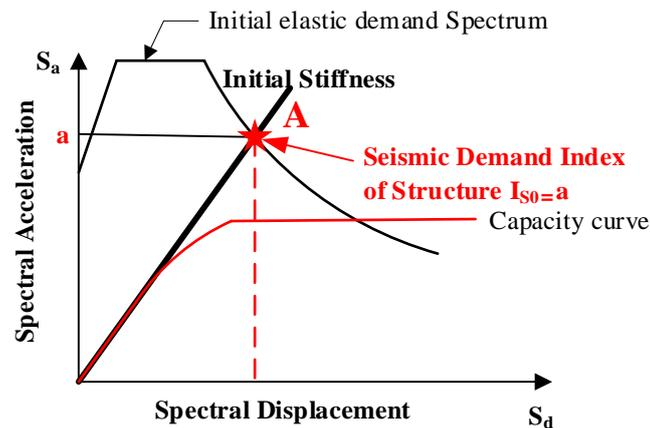
Fig. 4- Seismic Demand Index of Structure:  $I_{S0}$
