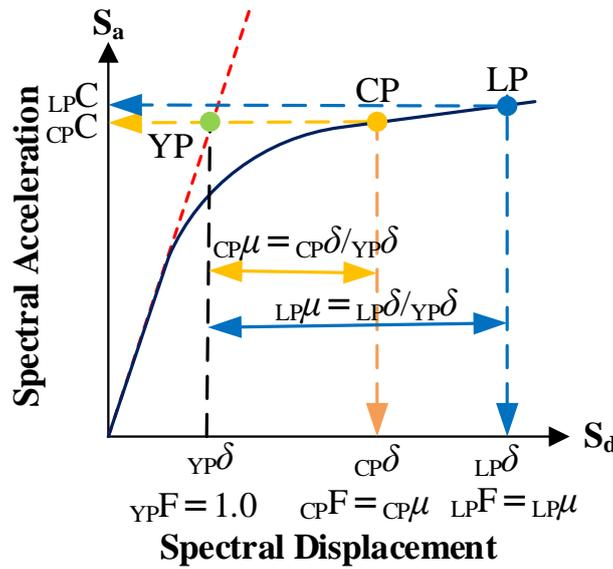
Fig. 5 – Evaluation of C index and F index by CP point and LP point
