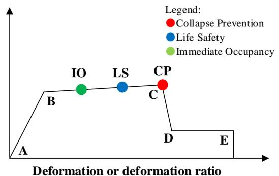
Fig. 3 –Acceptance Criteria for Nonlinear Procedures-Structural members (ATC40, ASCE41)
