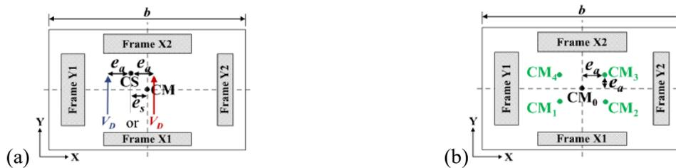
Figure 1. Conventional torsion design approaches: (a) Equivalent lateral force (static) analysis and (b) Dynamic analysis
