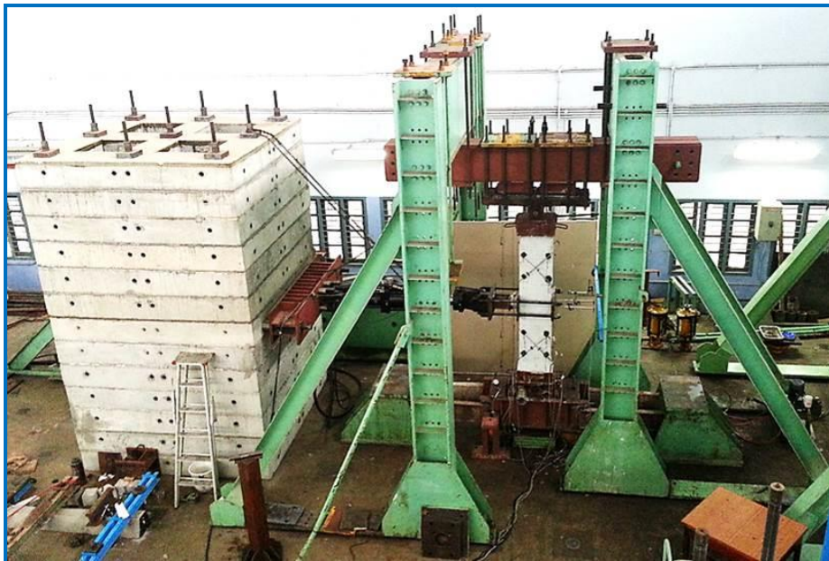
Fig. 2 – Test set-up showing a specimen under simultaneous lateral load and axial compression
