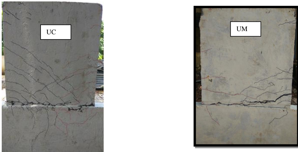
Fig. 10 –Crack Pattern for Specimen UC and UM
