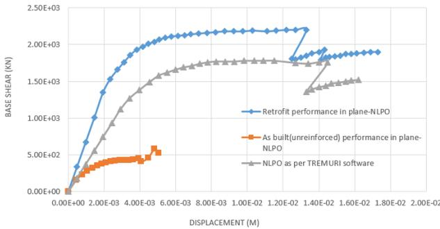
Fig.9- Pushover curve in X direction
