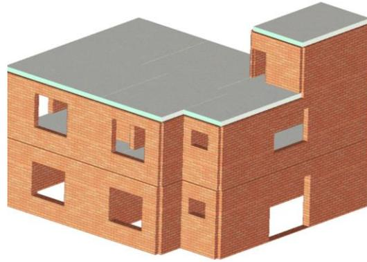
Fig.7- Model of the building in TREMURI Software
