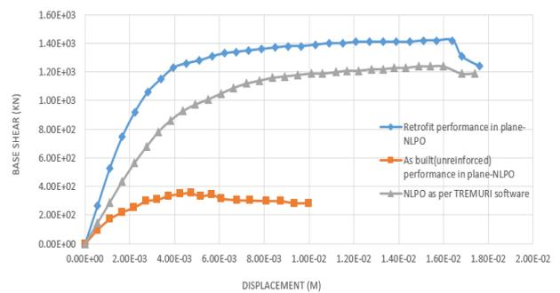
Fig.10- Pushover curve in Y direction
