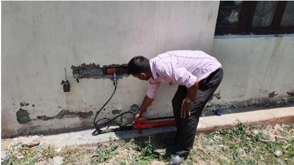
Fig. 3- Conducting In-situ Shear Test on Wall
