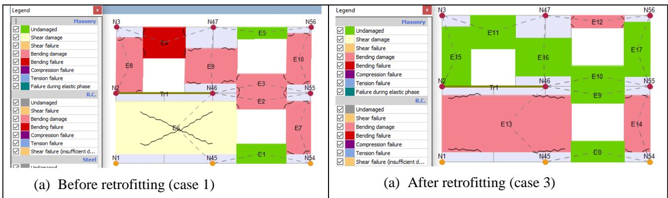
Fig.8- Progressive failure of wall (Grid 5-5) before and after retrofitting (TREMURI Software)
