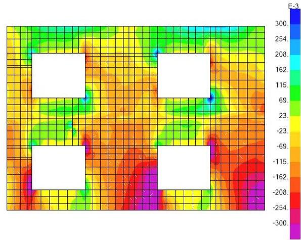
Fig.6- Compressive/Tensile stress (In plane stress (S22)) (Grid A-A)
