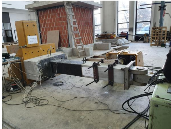
Fig. 9 - Quasi-static testing of the column models-MODEL M1.
