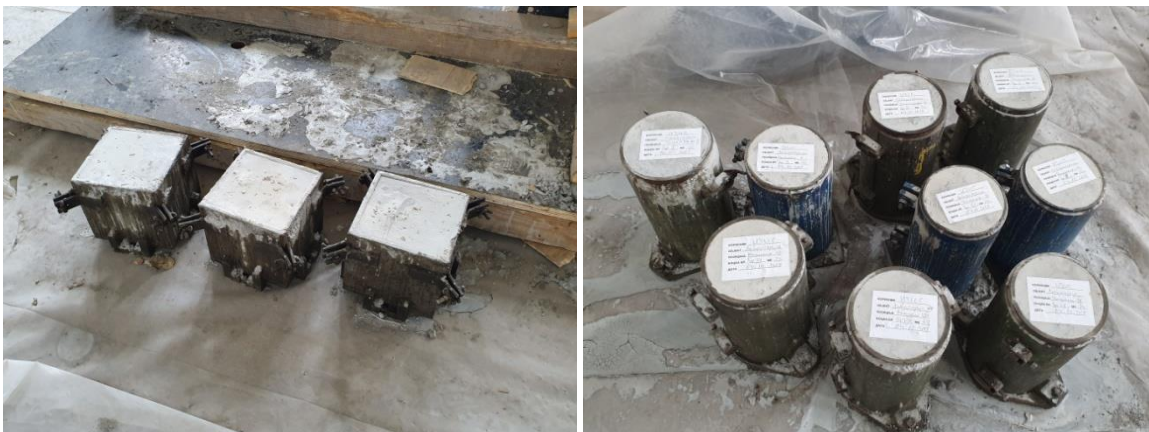
Fig. 2 - Photos of taken trial concrete specimens (cubes and cylinders).
