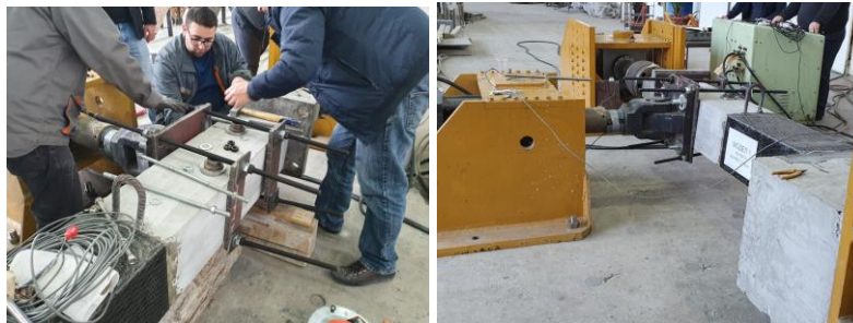
Fig. 8 – Assemblage of steel joints for application of forces and equipment for experimental tests.
