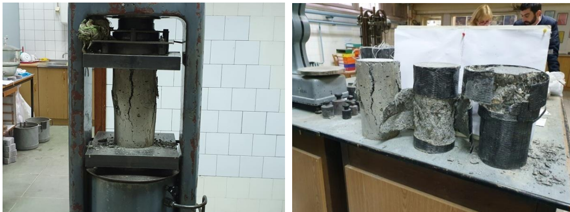
Fig. 4 - Testing of compressive strength for the three series.
