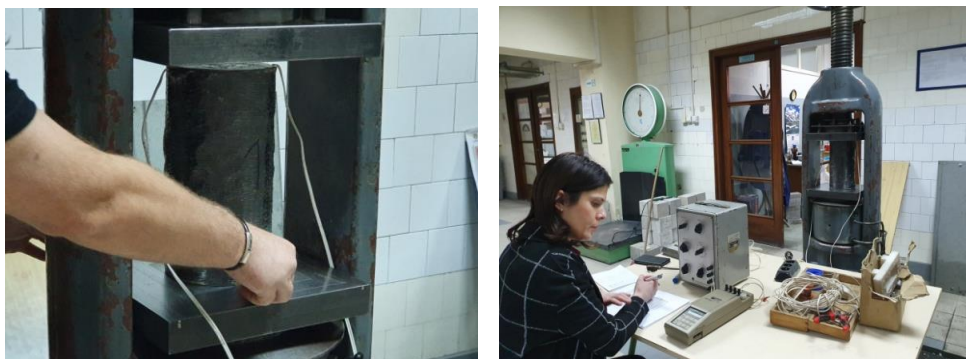
Fig. 5 - Testing of the static modulus of elasticity of all three series.
