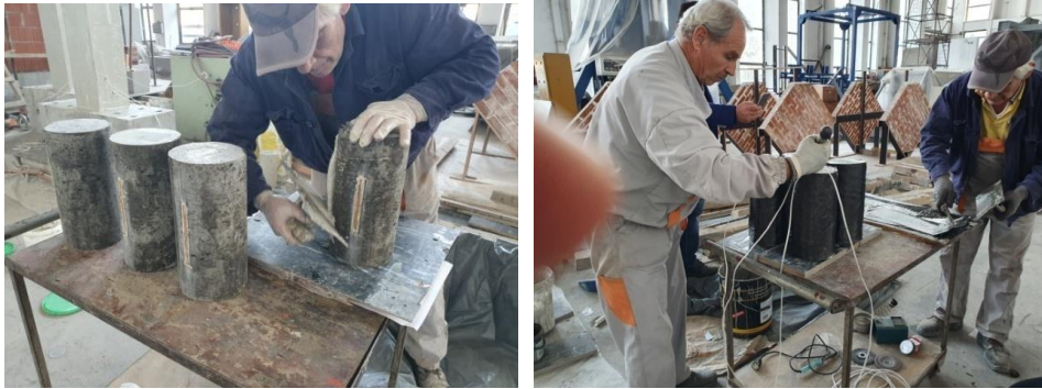
Fig. 3 - Preparation of trial concrete cylinders for testing.
