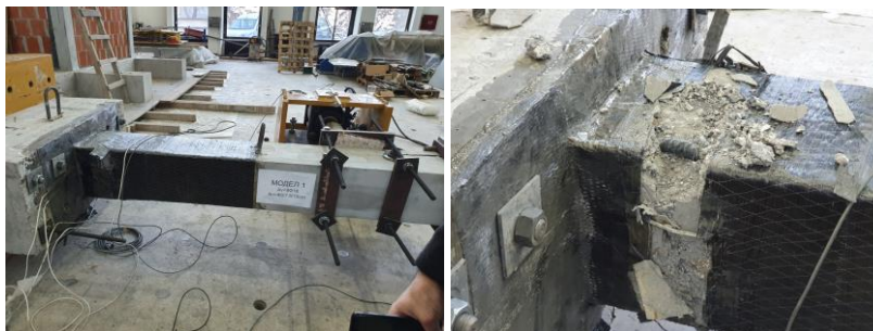
Fig. 10 shows some of the photos shot during quasi static testing of column Model M1.
