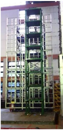
Fig. 6 A photo for an eight-story steel frame under shaking table tests
