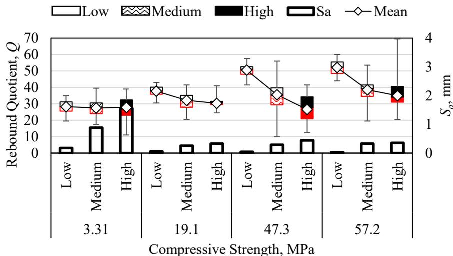
Fig.4 – Comparison of mean rebound quotient according to lower to higher compressive strength of concrete
