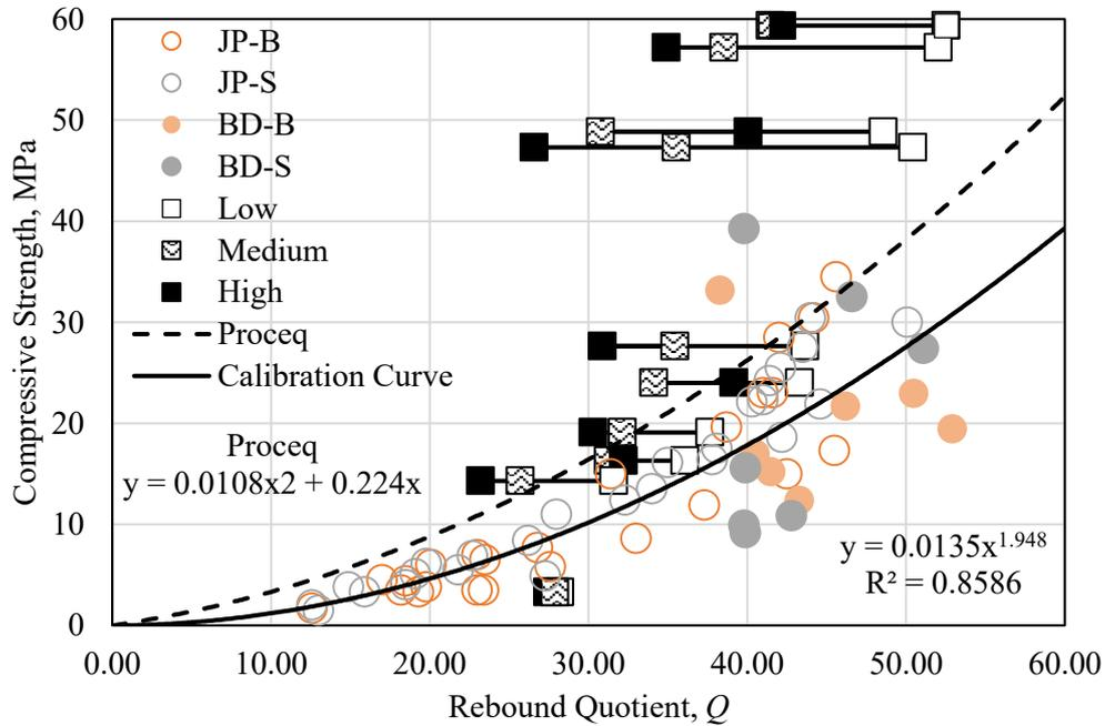
Fig. 5 – Comparison of mean rebound quotient  $Q$  on three types of surfaces of different roughness with developed calibration equation
