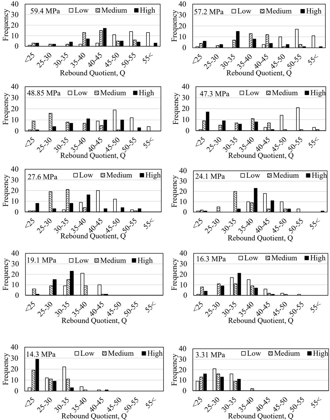
Fig. 3 – Results of rebound quotient Q depending on various degree of roughness
