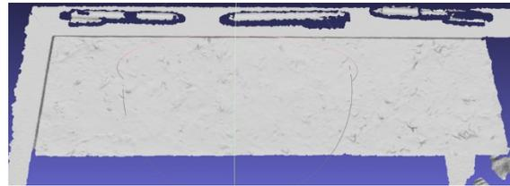
(d) Actual surface and recorded image with 3D scanning device for medium degree of roughness
