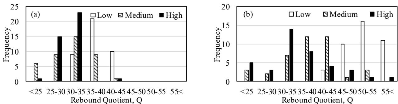
Fig 1. Variation of effect of surface roughness on different compressive strength levels of concrete. (a) Concrete compressive strength 19.1 MPa; (b) Concrete compressive strength 57.2 MPa.
