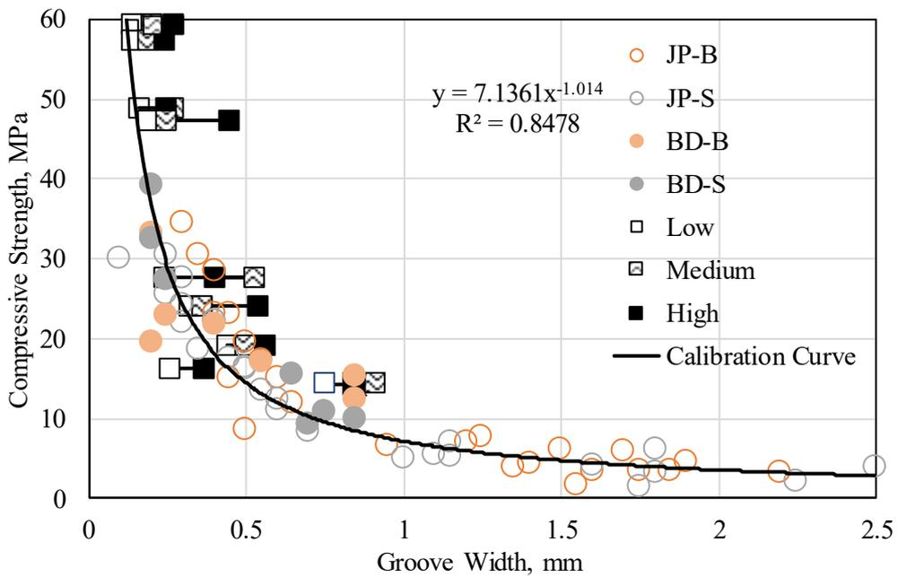
Fig. 6 – Comparison mean groove width (GW) on three types of surfaces of different roughness with developed calibration equation
