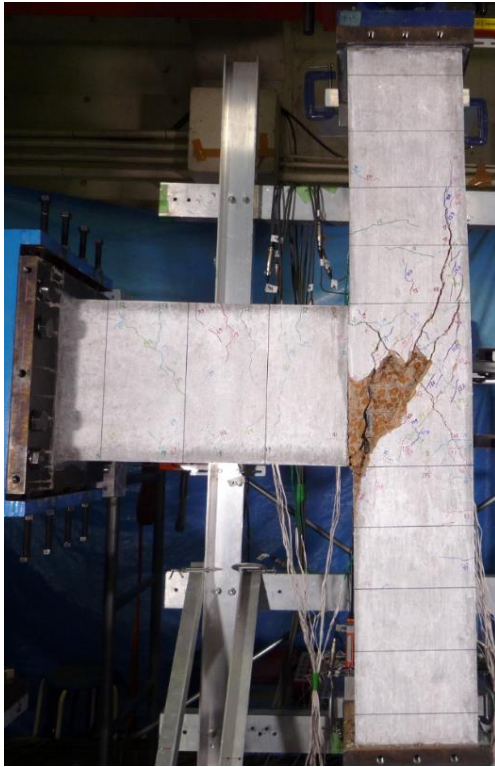
Fig. 4 – Damage to the specimen J1
