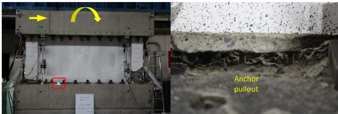
(a) (left) Overview of positive loading of Wall A, (right) showing pullout of anchors.
