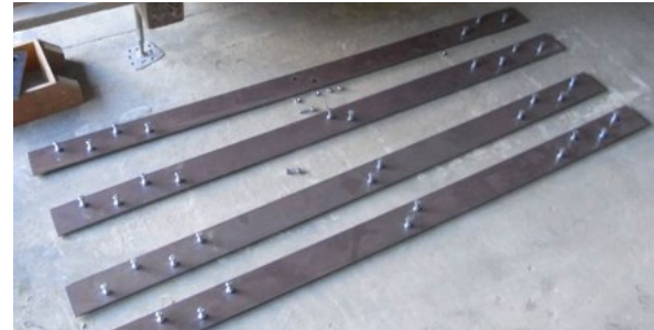
Fig. 4 – Installation of studs
