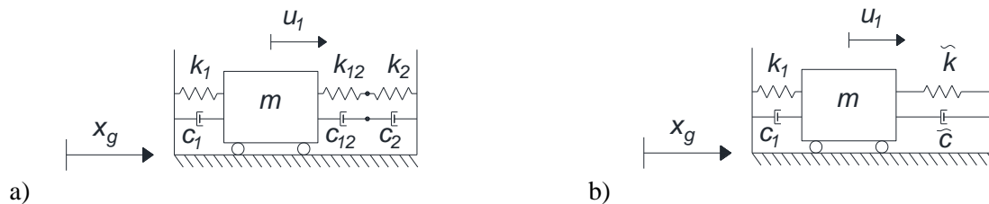
Fig. 2 – a) Simplified SDOF system; b) Simplified SDOF system with equivalent spring and damping.
