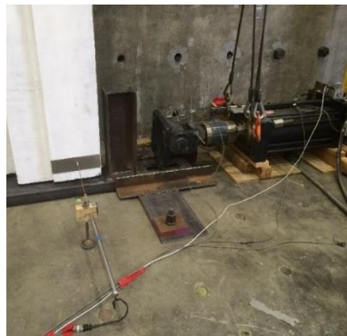
Setup for in-plane test with loading rail
