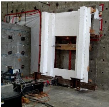
Setup for out-of-plane test
