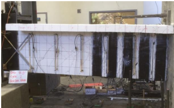
Fig. 8 –Setup of Specimen 3 (batten/groove strengthening at end) testing & force-deflection curve
