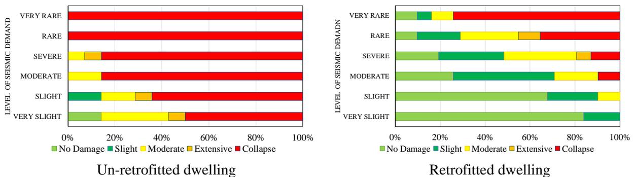
Fig. 11 – Damage level in dwellings with wall density of 2.9%
