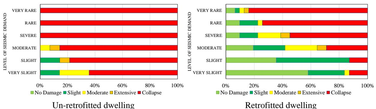
Fig. 9 – Damage level in dwellings with wall density of 1.7%
