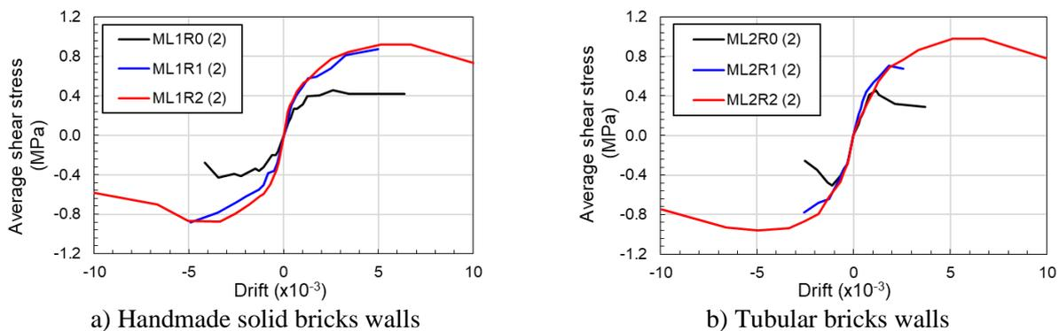
Fig. 7 – Capacity curves in terms of average shear stress and drift
