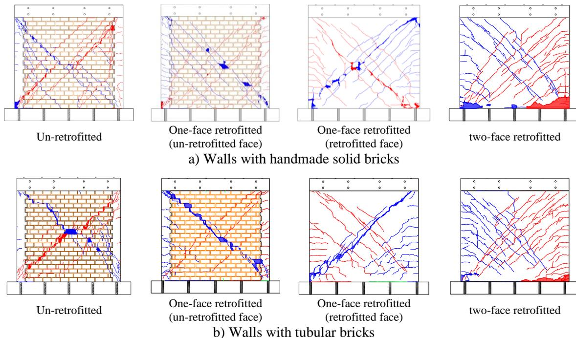
Fig. 8 – Ultimate state of walls with tubular bricks
