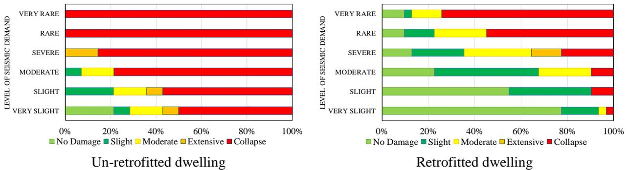
Fig. 10 – Damage level in dwellings with wall density of 2.3%
