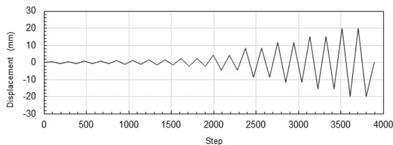
Fig. 3 – Loading displacement for lateral cyclic loading tests
