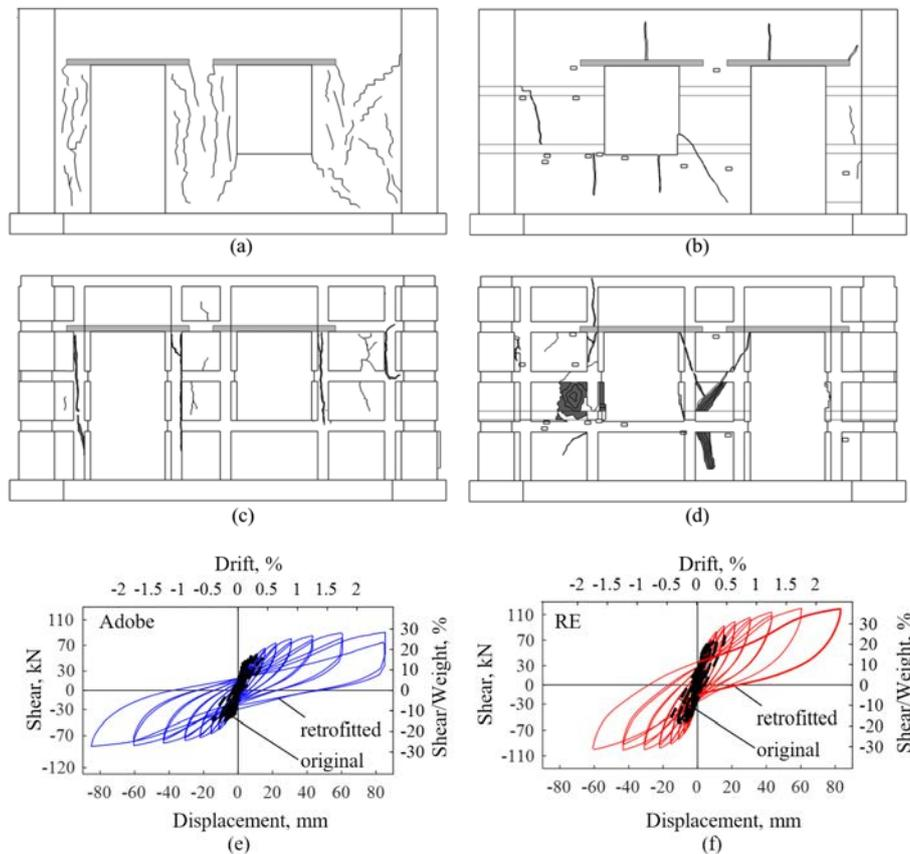
Fig. 6 – Representative results for Group 3 specimens. Cracking patterns of walls with openings: a) adobe wall bare 0.46% drift, b) RE wall bare 0.46% drift, c) adobe wall retrofitted 2.5% drift, d) RE wall retrofitted 2.5% drift. Cyclic response of: e) adobe specimens and f) RE specimens.
