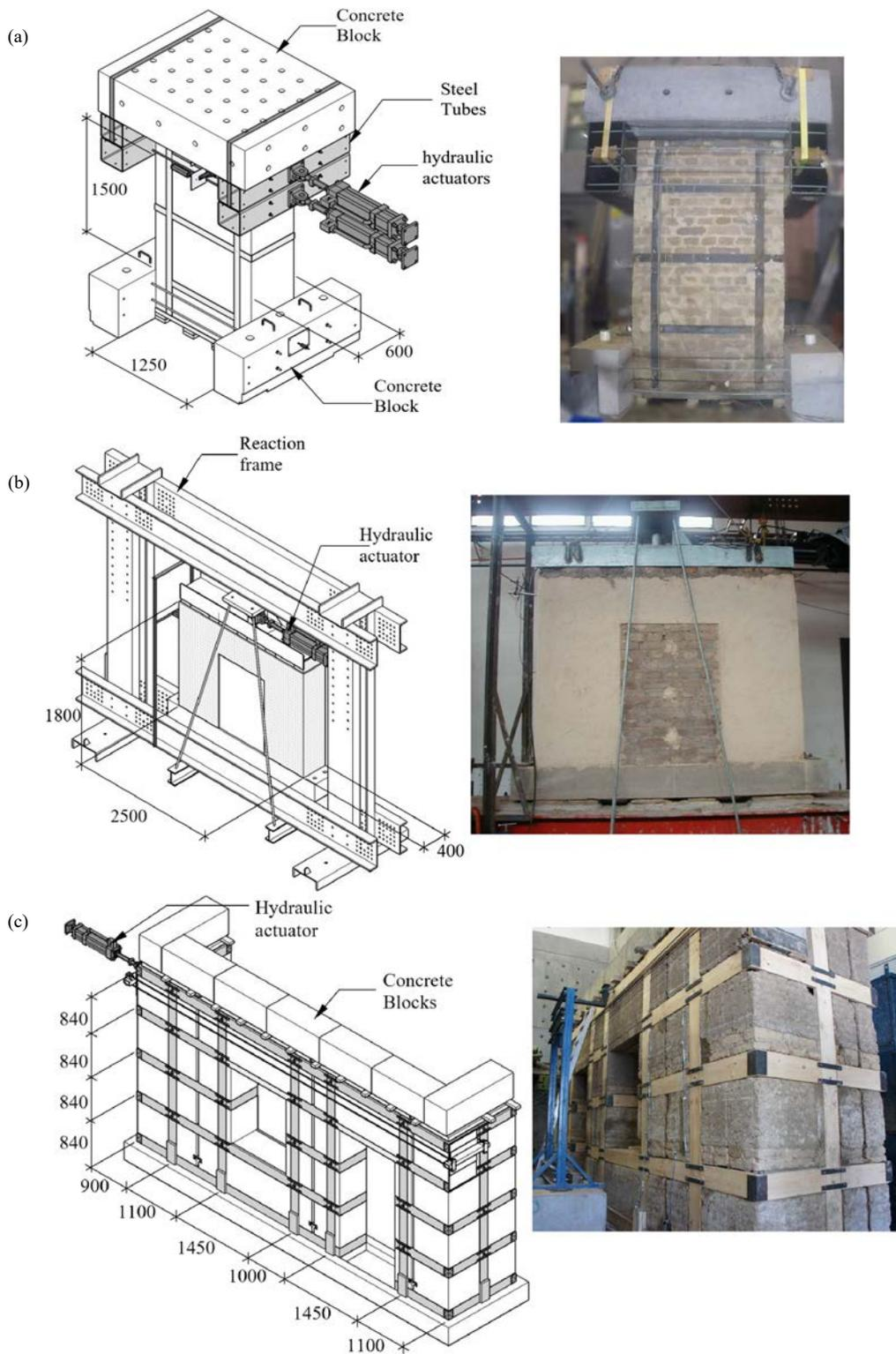
Fig. 1 – Test setup (unretrofitted counterparts not shown): (a) wall pier between window and door (Group 1); (b) wall pier between doors (Group 2); (c) wall façade with openings (Group 3).
