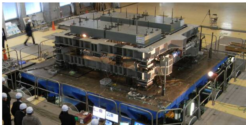
Photo 1 – Shaking table test situation
