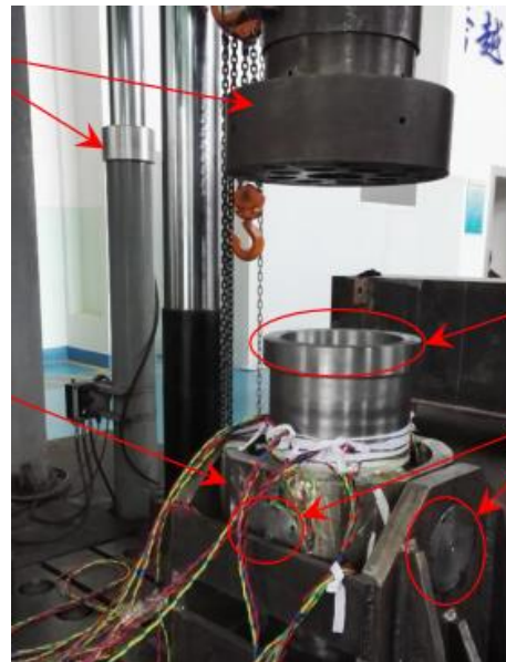
Fig. 7 Experimental test of middle supported joint of ODS
