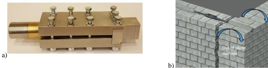
Fig. 5. Friction-based Dissipative device proposed by D’Ayala and Paganoni, b) insertion of dissipative anchoring system at the connection between orthogonal walls.
