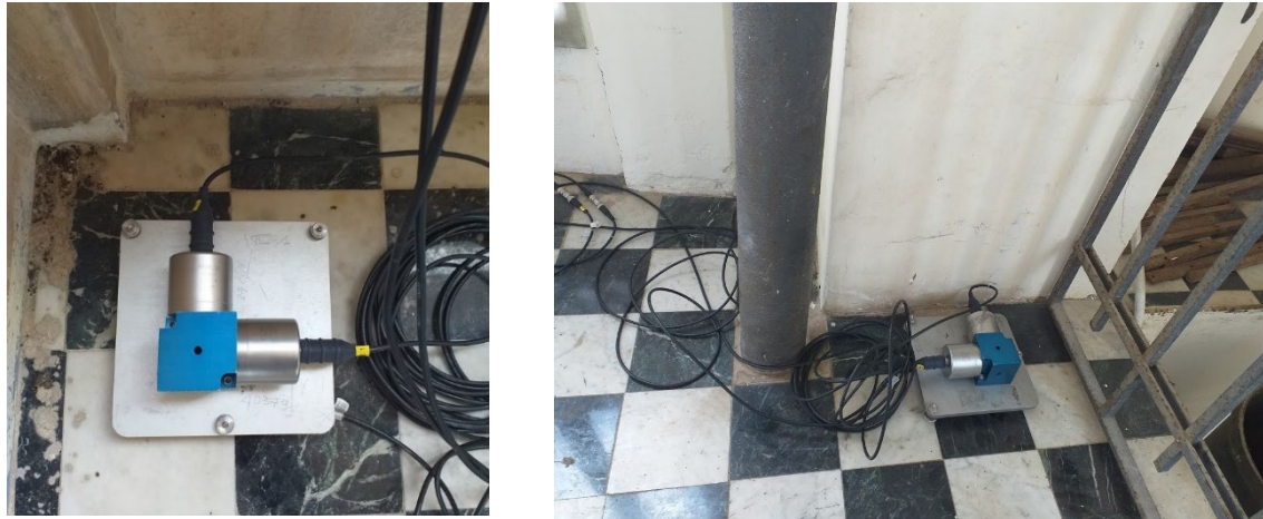
Fig. 3 – Accelerometers used in the environmental noise measurement
