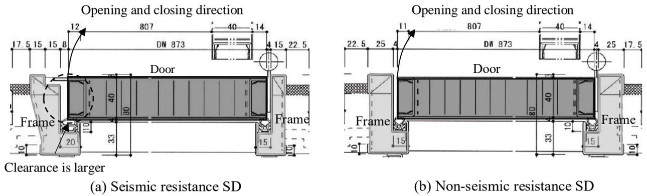
Fig. 5 – Cross section of the SDs
