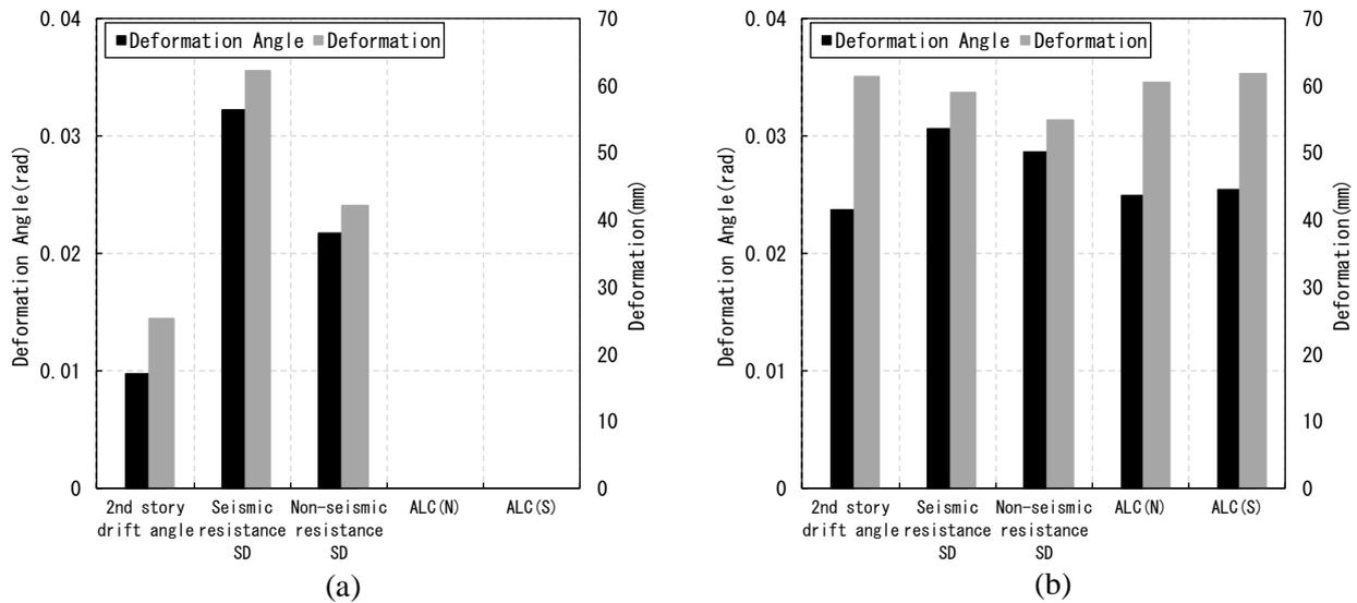
Fig. 21 – Maximum story drift angle of the 2<sup>nd</sup> story and the maximum in-plane deformation angles of the SDs and ALC panels in the (a) wall direction and (b) frame direction
