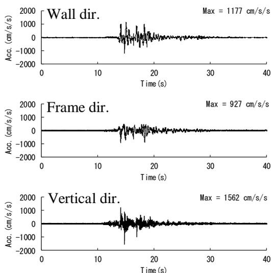
Fig. 15 – Floor response acceleration on the 2<sup>nd</sup> story
