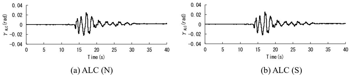
Fig. 20 – Time histories of the in-plane deformation angle of the ALC panels
