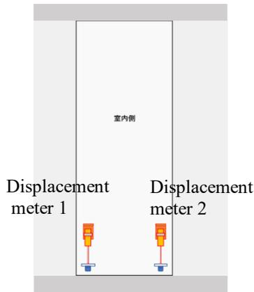
Fig. 9 – Measurement method of the in-plane deformation angle of the ALC panel
