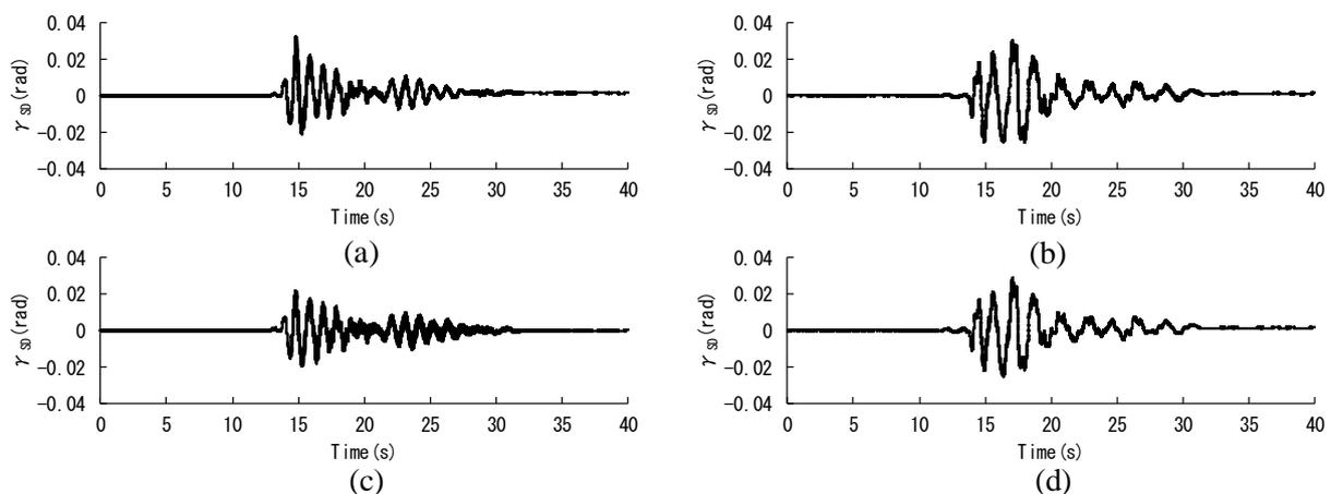
Fig. 19 – Time histories of the in-plane deformation angle of the seismic resistance SD (a) in the wall direction and (b) in the frame direction and the non-seismic resistance SD (c) in the wall direction and (d) in the frame direction
