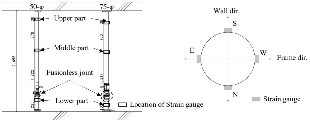
Fig. 14 – Attachment locations of strain gauges
