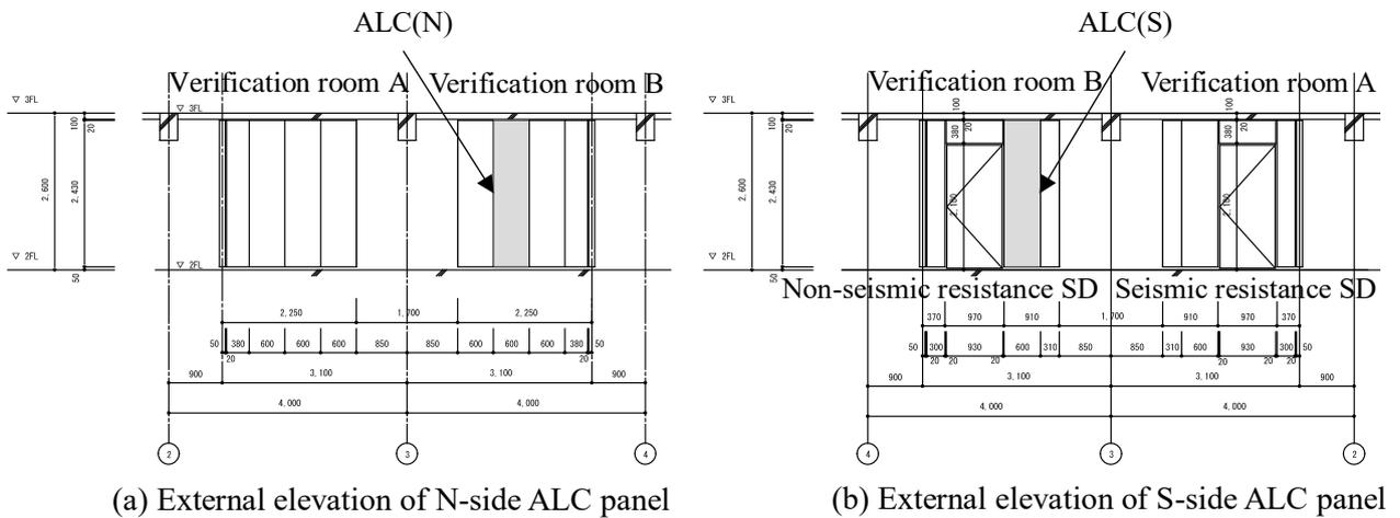
Fig. 6 – Elevation view of the ALC panels
