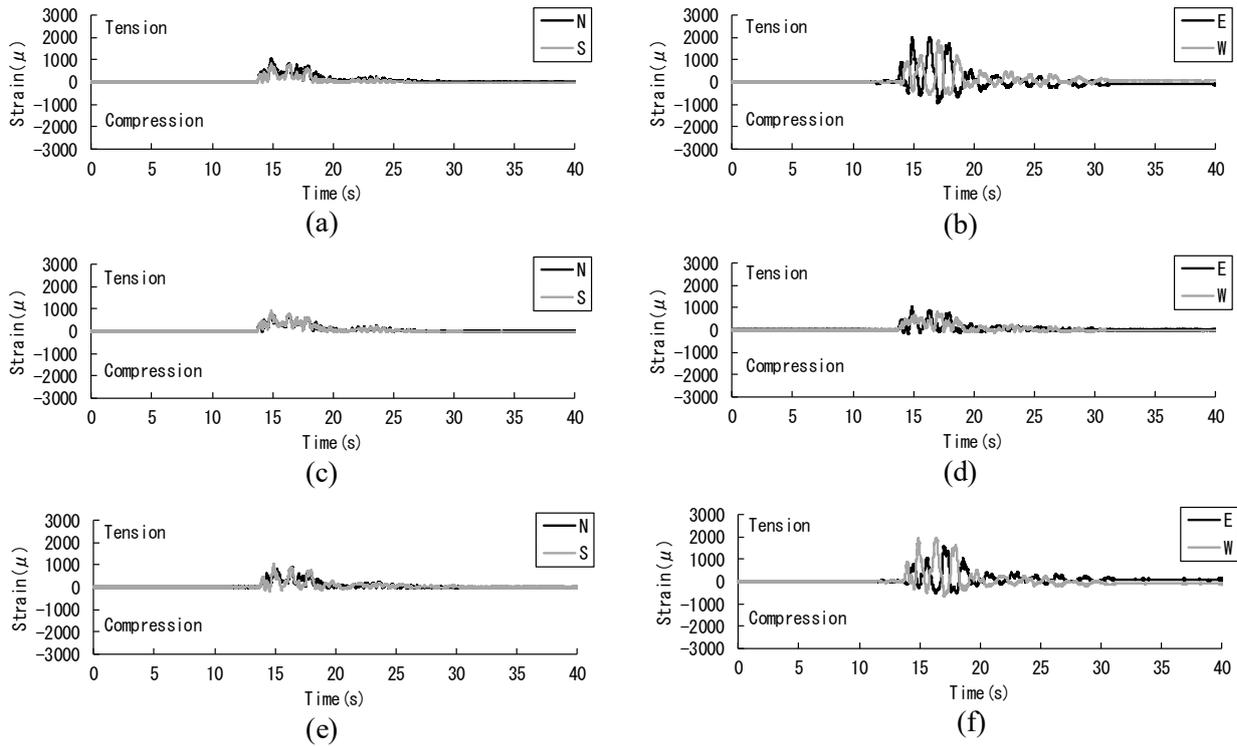
Fig. 24 – Time histories of the strain on water supply vertical pipe of 50- $\phi$  in the upper part (a) in the wall direction and (b) in the frame direction, in the middle part (c) in the wall direction and (d) in the frame direction, and in the lower part (e) in the wall direction and (f) in the frame direction
