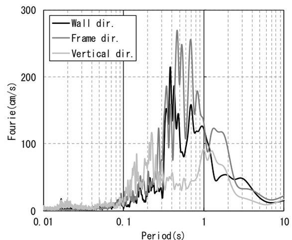
Fig. 16 – Fourier spectra of floor vibration on the 2<sup>nd</sup> story
