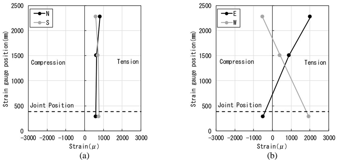
Fig. 25 – Strain distribution at the time of the maximum story drift angle of the 2<sup>nd</sup> story (a) in the wall direction and (b) in the frame direction
