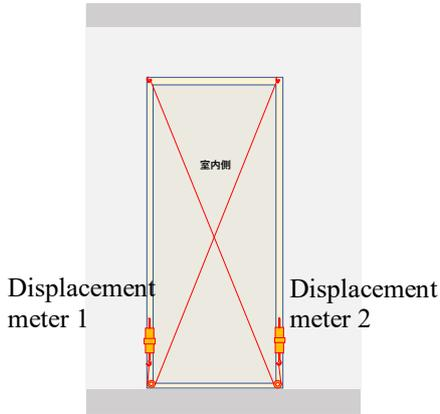
Fig. 7 – Measurement method of the in-plane deformation angle of the SD
