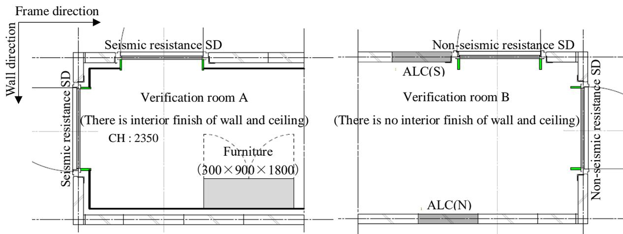
Fig. 3 – Rough plan of the verification rooms
