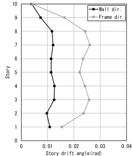
Fig. 17 – Displacement meters for measuring story drift angle Fig. 18 – Maximum story drift angle [2]
