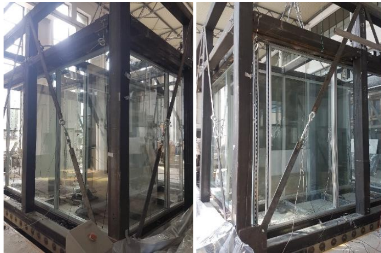
Fig. 8 Partition wall systems on the shake table (configurations 3 and 4)
