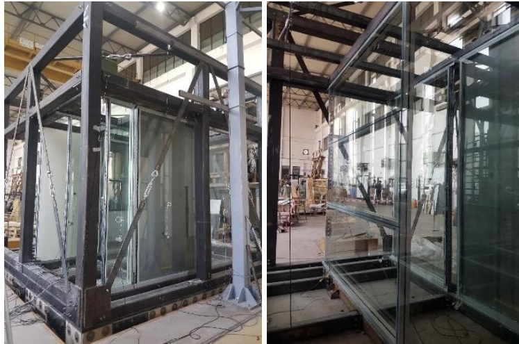
Fig. 7 Partition wall systems on the shake table (configurations 1 and 2)
