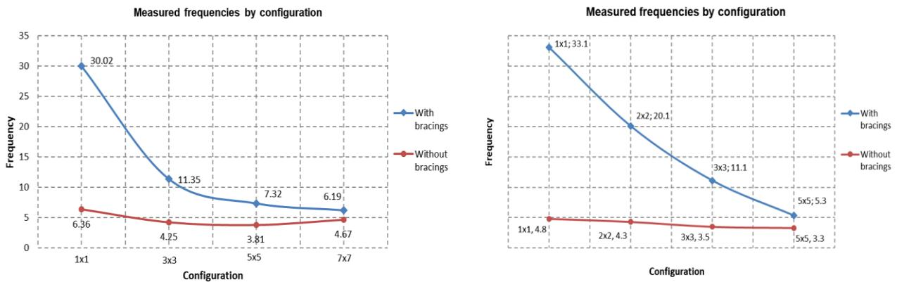
Fig. 4 – Change of dynamic characteristics of raised floors (left 1.0m high, right 1.5m high)
