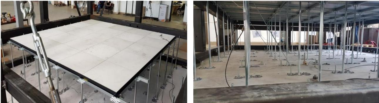
Fig. 2 – Five by five panel configuration – left. Raised floor structure – right.
