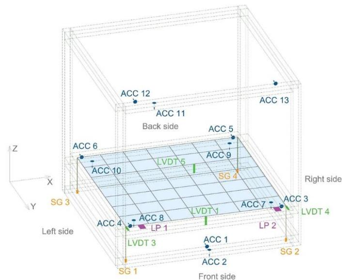
Fig. 3 – Instrumentation set up for a raised floor system
