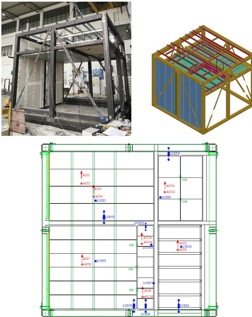
Fig. 7 – Ceiling systems - test setup and instrumentation.
