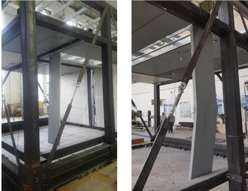
Fig. 10 – Damaged panels
