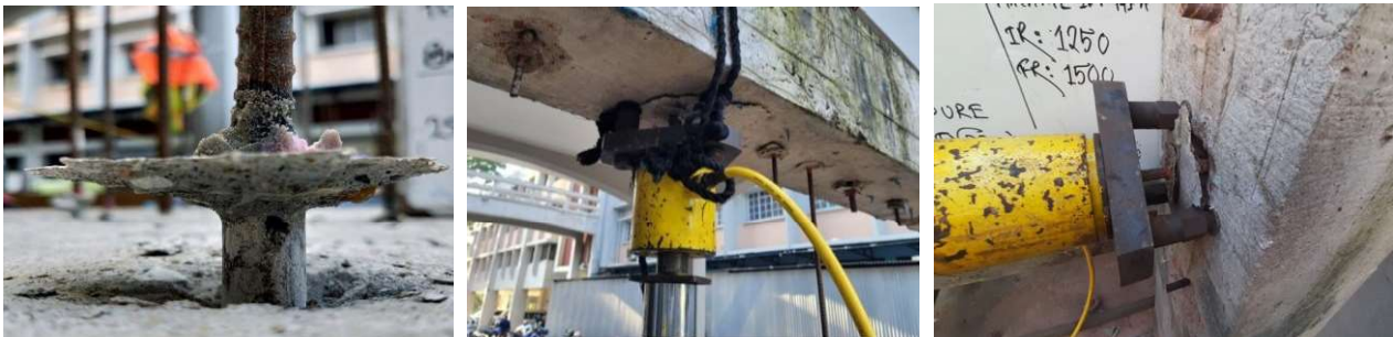
Fig. 6 – Typical Failure patterns of anchor bars observed during experiment
