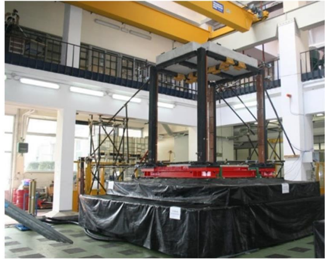
Fig. 3 – (a) 3D structural model of the base-isolated structure, (b) small scale building on RR-FRBs tested at the University of Naples [7].
