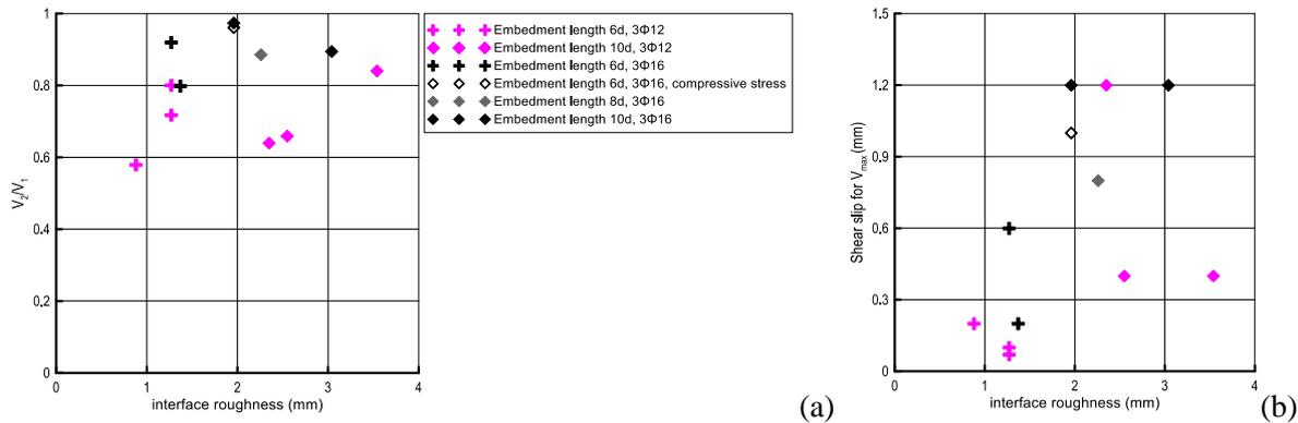
Fig. 8- (a) Reduction of the resistance during cycling, (b) Value of the shear slip at which the maximum interface resistance is mobilized, as a function of the roughness of the interface for various embedment lengths of the post-installed reinforcing bars.
