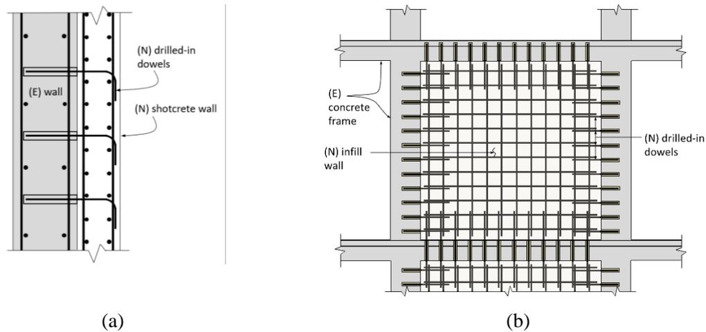
Fig. 2 – (a) Seismic strengthening with an onlay shear wall; (b) Frame retrofit with infill shear walls
