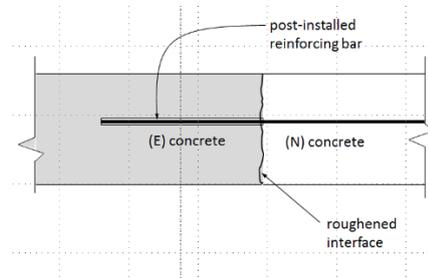
Fig. 1 – Post-installed reinforcing bars
