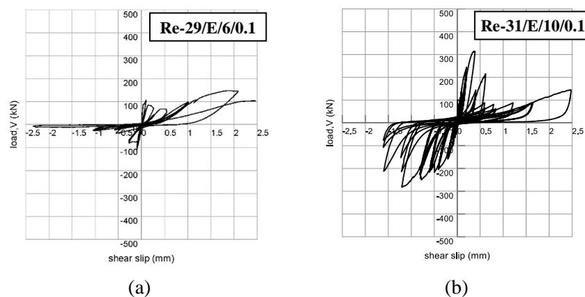
Fig. 5- Typical hysteresis loops for specimens reinforced with 12mm bars, having embedment equal to (a)  $6d_b$  and (b)  $10d_b$ .
