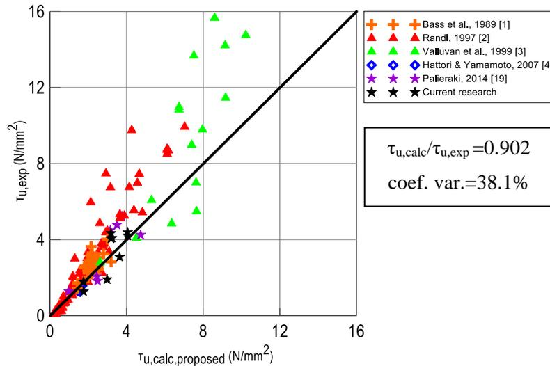
Fig. 9- Interfaces crossed by post-installed reinforcing bars; Comparison between experimental shear resistance and values calculated based on the proposed formula.
