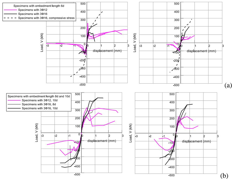
Fig. 7- Hysteresis loop envelopes for specimens with  $3\Phi 12$  or  $3\Phi 16$  reinforcing bars, with embedment length of the bars (a)  $6d_b$  and (b)  $8d_b$  or  $10d_b$ : first cycle and third cycle.
