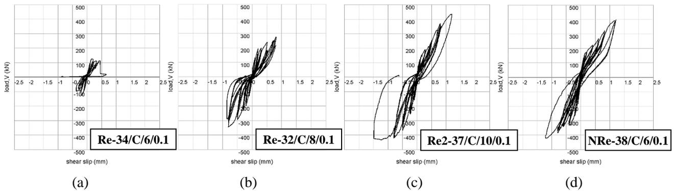
Fig. 6- Typical hysteresis loops for specimens reinforced with 16mm bars, having embedment equal to (a)  $6d_b$ , (b)  $8d_b$ , (c)  $10d_b$ , (d)  $6d_b$  and compressive stress perpendicular to the interface.
