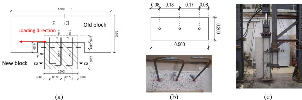
Fig. 4- (a) Geometry of specimens (b) Interface reinforcement and photo of roughened interface, with the reinforcement positioned, before concreting the block simulating the new part of concrete (c) Test setup and specimen in testing position
