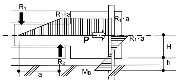
Fig. 3 – Assumption of moment diagram in the elastic range
