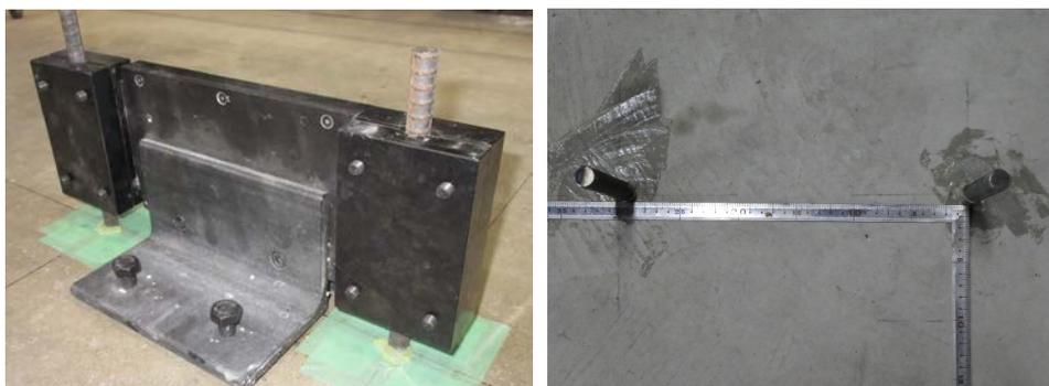
Fig. 22 – Installation of test anchor bars
