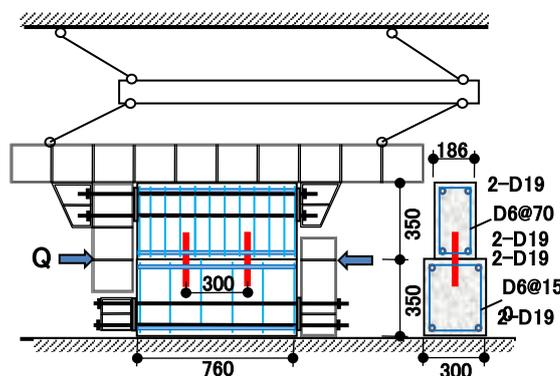
Fig. 11 – Loading apparatus for shear experiment in laboratory
