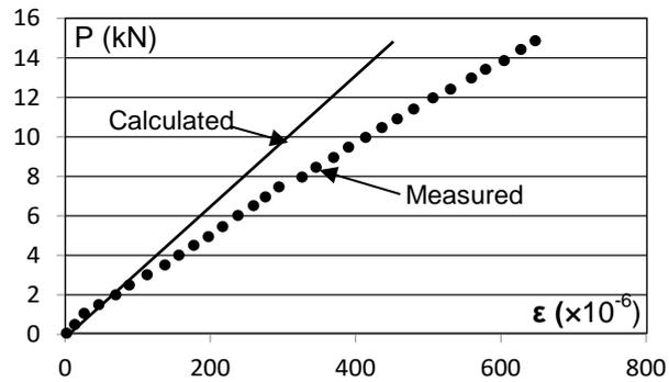
Fig. 4 – Calculated and measured edge strain of the convex base
