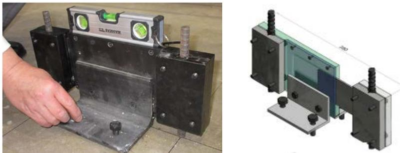
Fig. 21 – Setup of test anchor bars with an auxiliary anchor bar holding device
