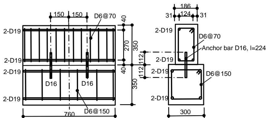
Fig. 12 – Test specimen
