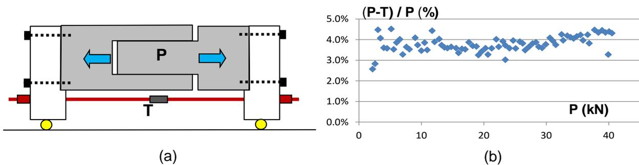
Fig. 7 – Measuring method of frictional force and measurement results
