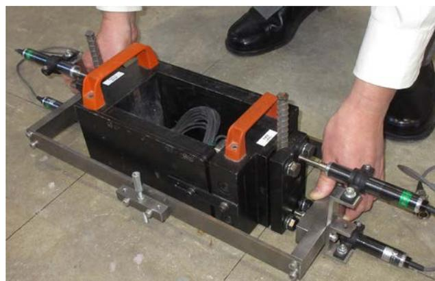
Fig. 24 – Setup of the gage holder
