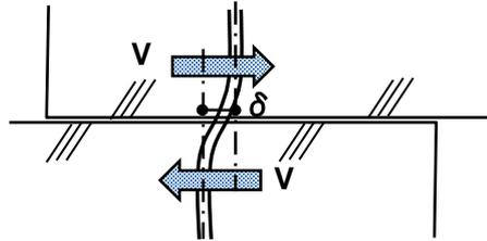
Fig. 1 – State of deformation of anchor bar on the concrete-concrete interface
