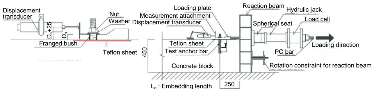
Fig. 16 – JCAA shear test method [2]
