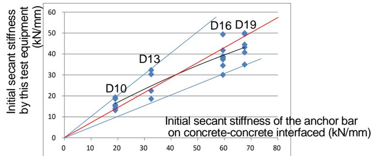
Fig. 15 – Initial secant stiffness
