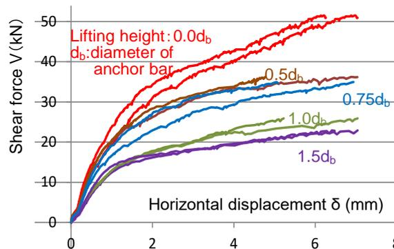
Fig. 10 – Relation between the horizontal load and displacement depending on the lifting height
