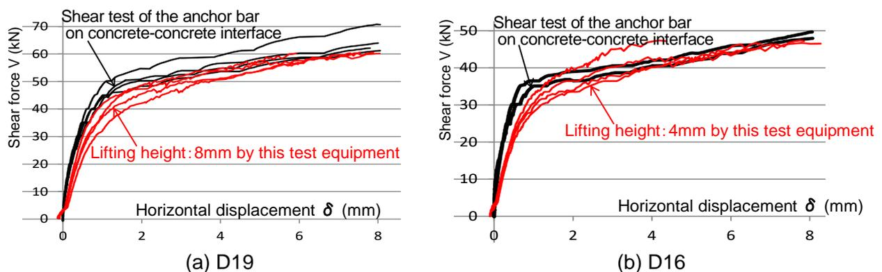
Fig. 14 – Relations between the shear force and the horizontal displacement
