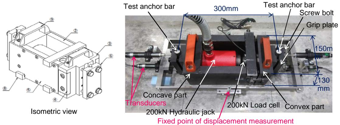
Fig. 6 – Feature of the test equipment
