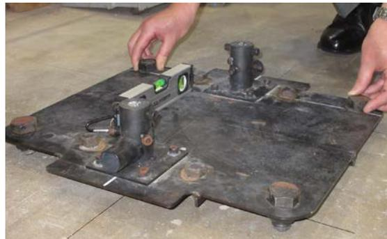
Fig. 19 – Setup of an auxiliary device for drilling
