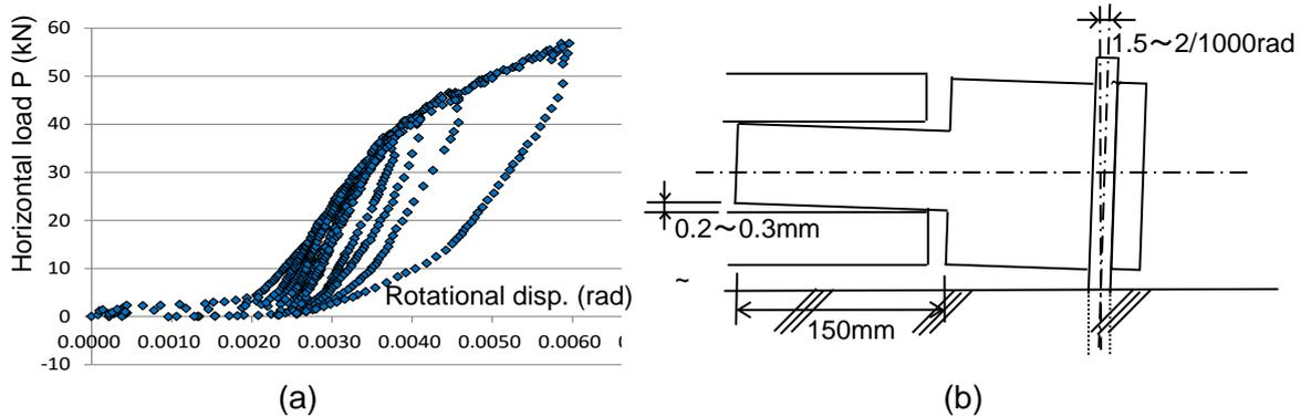
Fig. 8 – Example of the measured rotational displacement and the cause of the initial displacement
