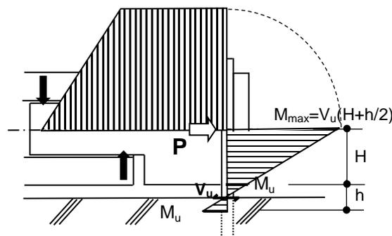
Fig. 5 – Assumption of moment diagram in the plastic range
