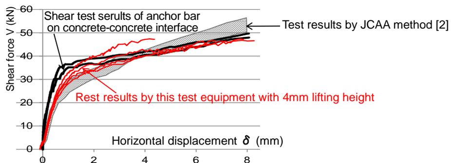
Fig. 17 – Comparison of the test by this test equipment with JCAA method [2]
