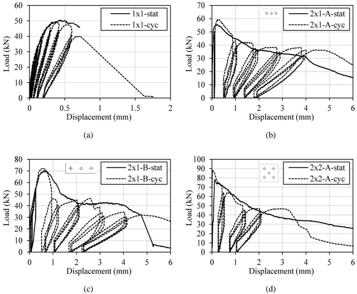
Fig. 3 – Typical load-displacement curves obtained from the tests on single anchors and anchor groups under static and cyclic loading (a) Single anchor, (b) 2x1-A configuration, (c) 2x1-B configuration, and (d) 2x2-A configuration
