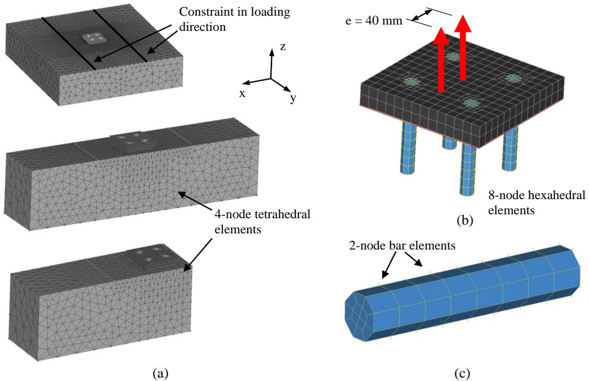
Fig. 5 – FE Models (a) Complete models, (b) Discretization of fixture and anchor rods, and (c) Anchor rod with 2-node bar elements for bond
