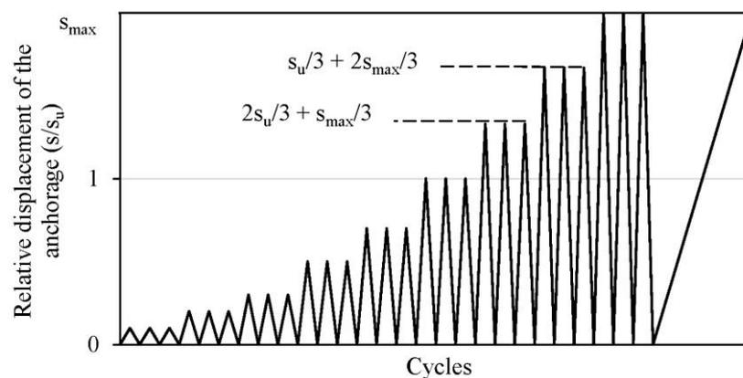
Fig. 2 – Schematic structure of the test procedure for displacement-controlled pulsating tension load
