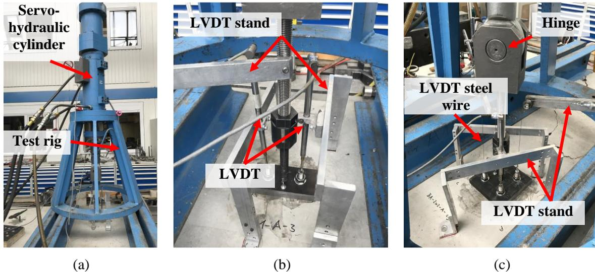
Fig. 1 – Experimental setup (a) Servo-hydraulic cylinder, (b) setup for 2 x 1 configuration, and (c) setup for 2 x 2 configuration
