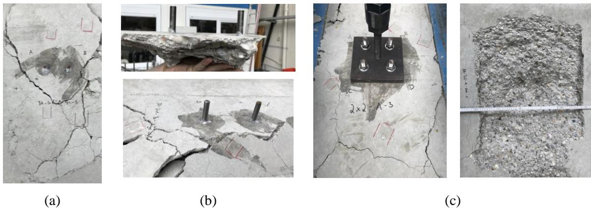
Fig. 4 – Typical failure modes (a) 2x1-A configuration, (b) 2x1-B configuration, and (c) 2x2-A configuration
