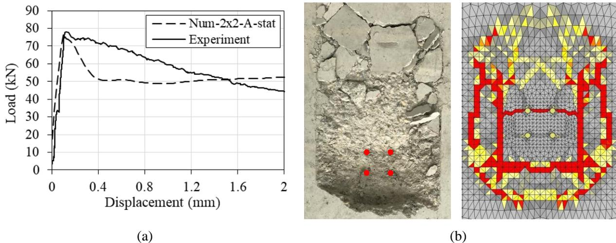
Fig. 6 – Comparison of experimental and numerical results for the 2 x 2 configuration (a) load-displacement curves (b) obtained crack pattern
