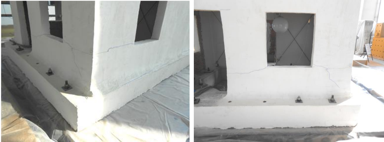
Fig. 6 - Damage of BM-SR model after final test, (left: S-E corner, right: South wall)
