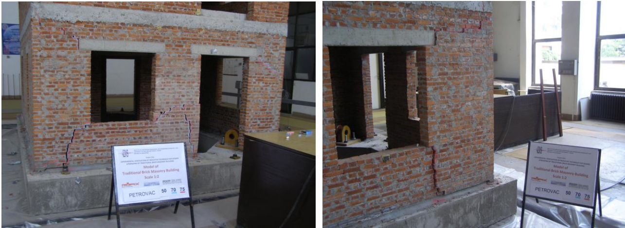
Fig. 4 – Damage to the model after final test ( acc_{max}=0.35g )
