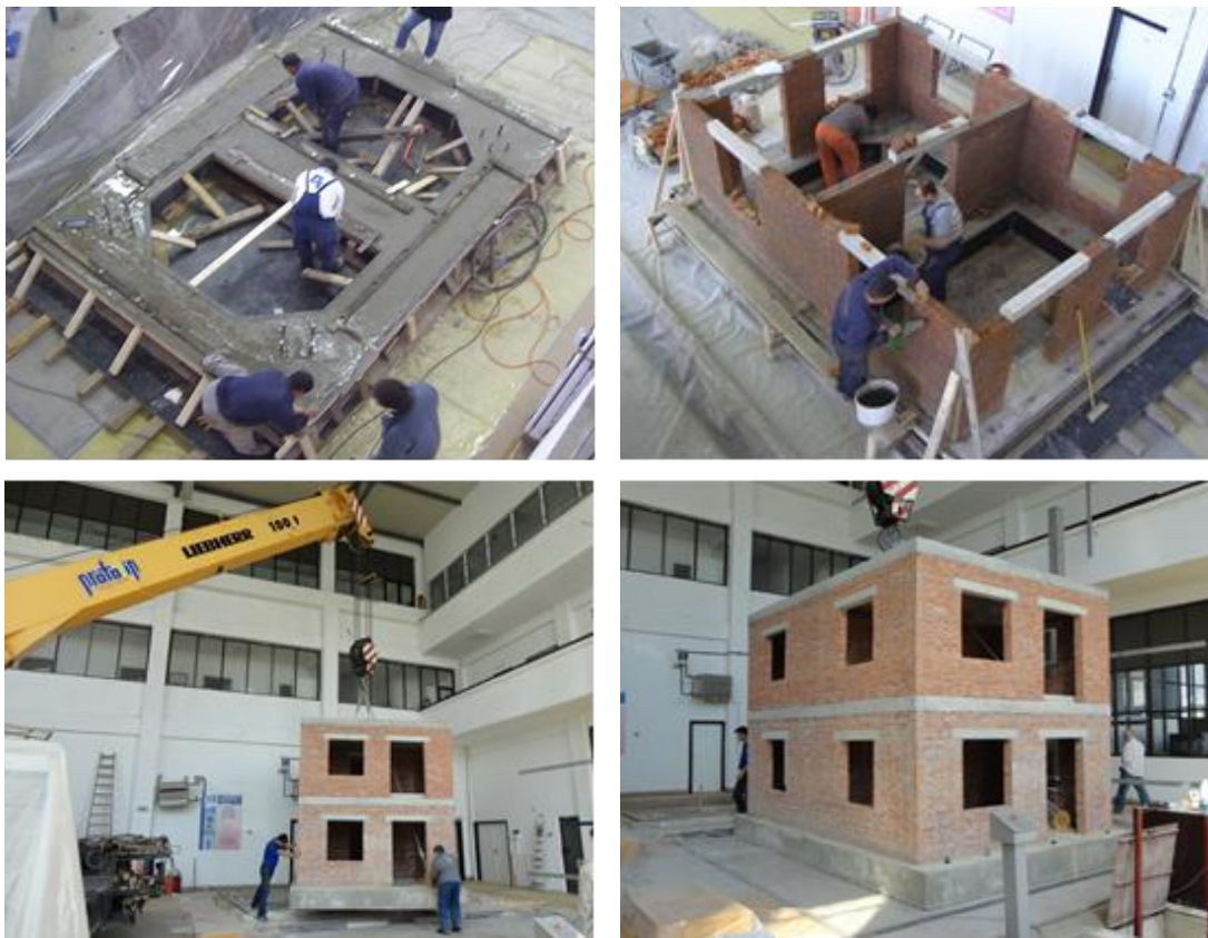
Fig. 2 - Construction and transportation of the brick masonry non-retrofitted model, BM
