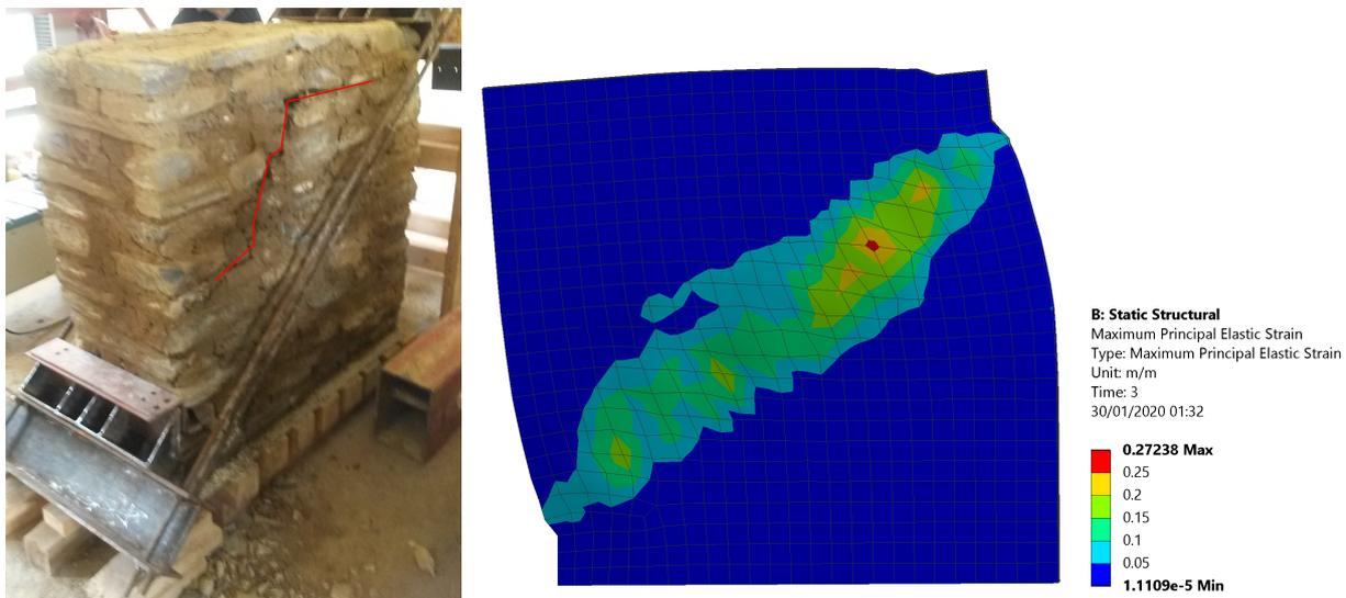
Fig. 10 – Experimental panel crack pattern (left) and numerically predicted crack pattern (right).
