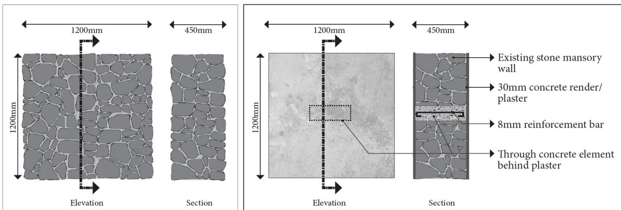
Fig. 2 – Relief of the different panels tested: existing SMM wall (left) and retrofitted SMM Wall (right).
