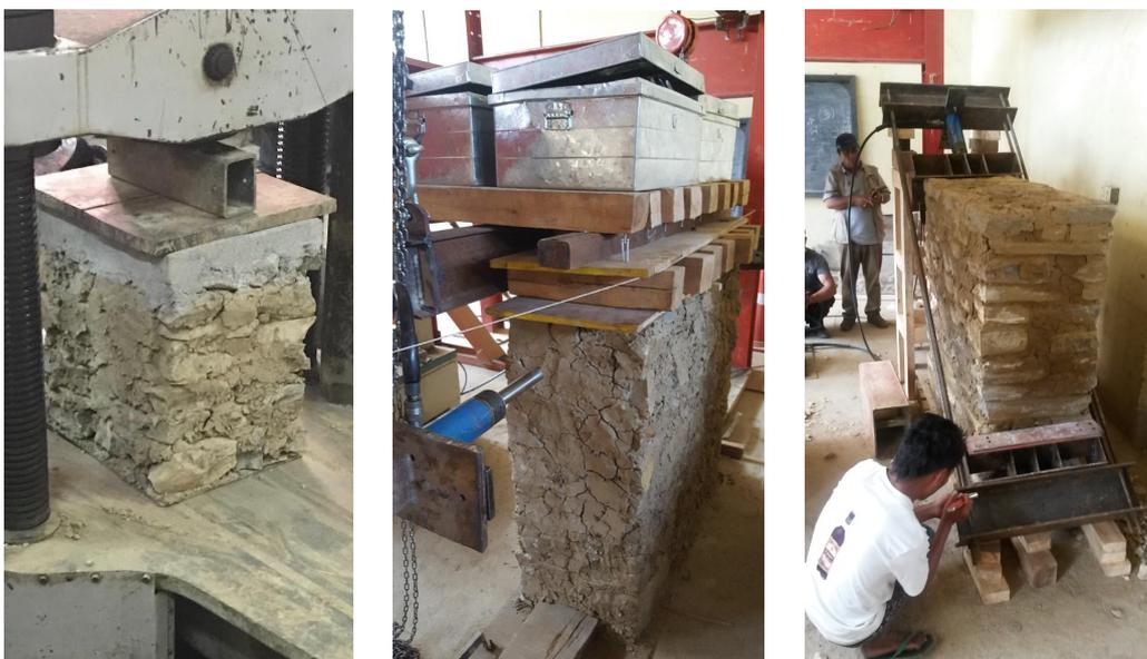
Fig. 3 – Uniaxial compression test setup (left), combined axial and shear test (middle) and diagonal compression test (right).
