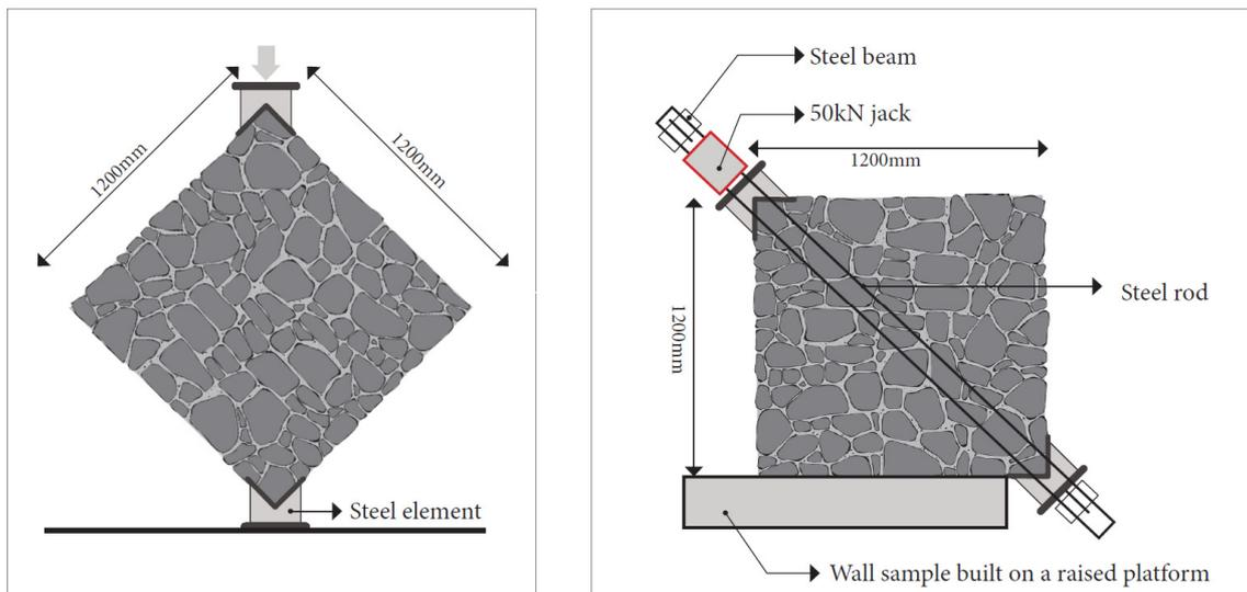
Fig. 5 – ASTM test setup (left) and revised setup (right).
