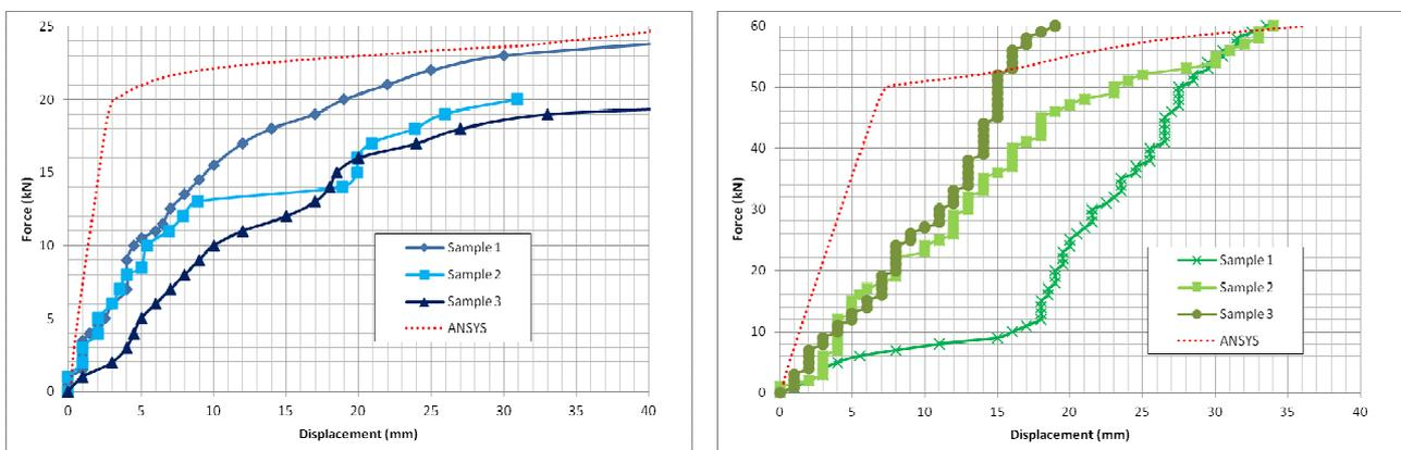
Fig. 9 – Experimental and numerical results for existing SMM panels (left) and retrofitted panels (right).
