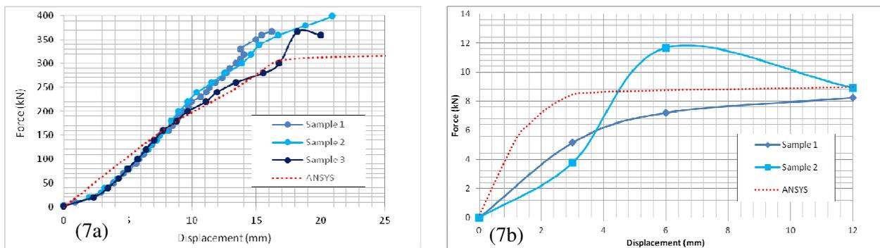
Fig. 7 – Comparison of the force-displacement plots between the experimental results and the numerical simulation output for the uniaxial compression test (a) and the combined axial and shear test (b).
