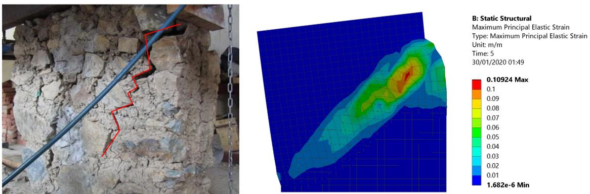
Fig. 8 – Similar failure/crack patterns between the experimental observations and the FEA model output.
