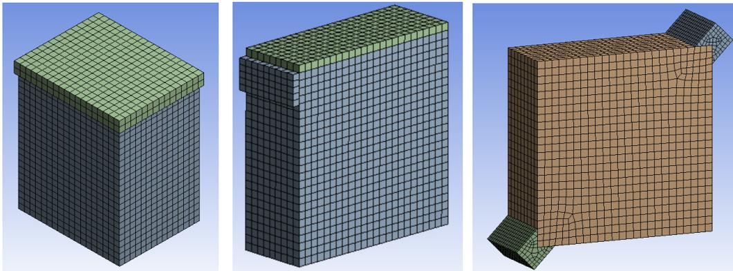
Fig. 6 – A finite element discretisation of the masonry panels used in the uniaxial compression test (left), combined axial and shear tests (middle) and diagonal compression test (right) numerical analyses.
