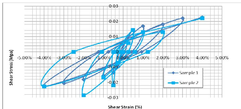
Fig. 4 – Shear Stress/Shear Strain experimental results for the two combined axial and shear test samples.
