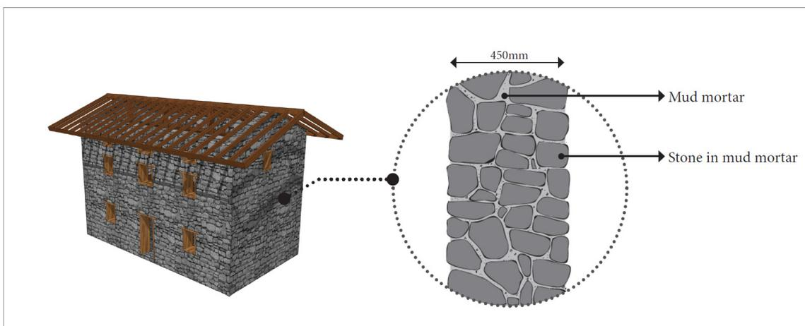
Fig. 1 – A typical traditional Nepalese house (left) and a section through a SMM wall (right).
