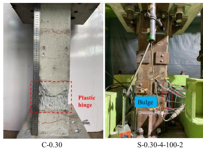
Fig. 12 – Failure modes
