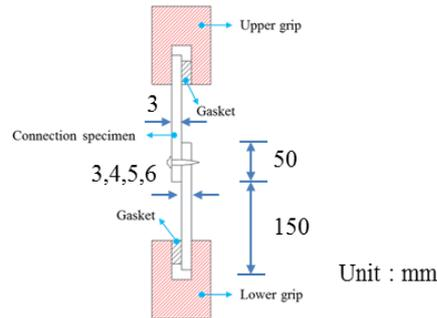
Fig. 4 – Assembly diagram of connection sample
