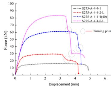
Fig. 6 – Shear load versus displacement of connections
