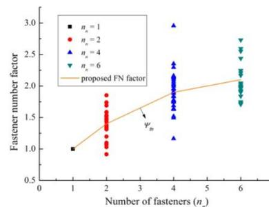
Fig. 10 – Factor depending on number of fasteners
