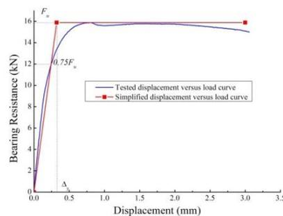
Fig. 8 – Simplified bilinear curve
