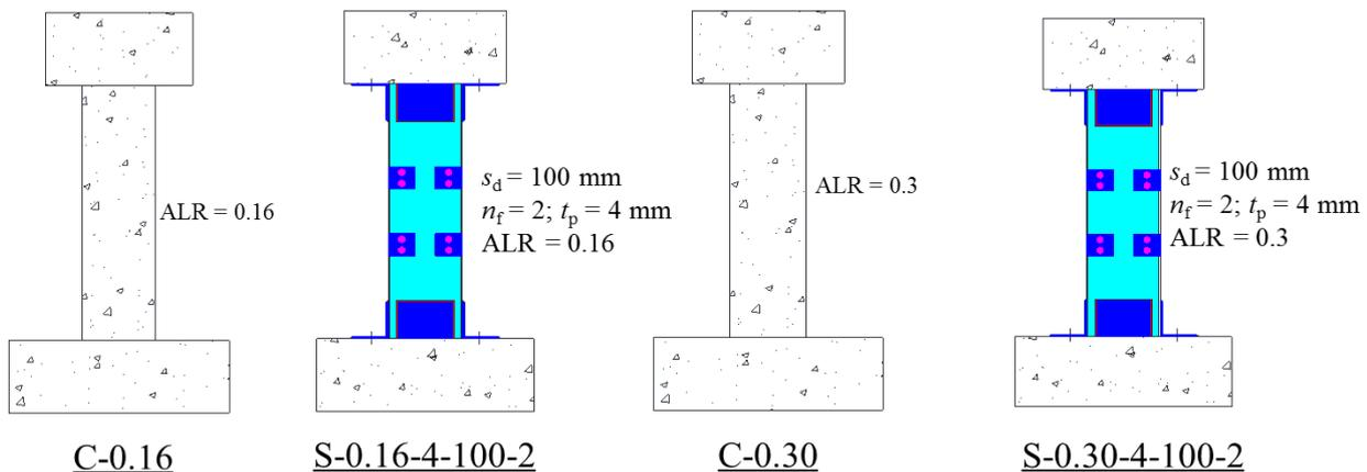
Fig. 11 – Configuration of tested samples
