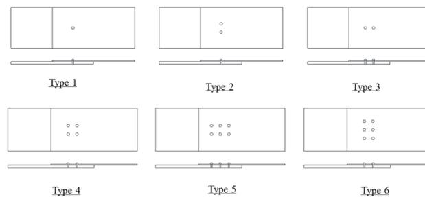
Fig. 2 – Configurations of tested specimens
