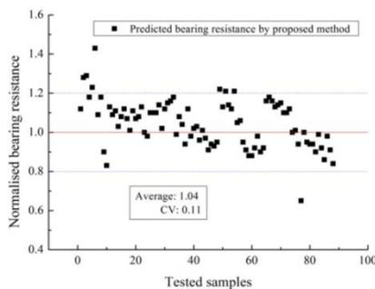
Fig. 7 – Comparison between predicted and measured peak loads
