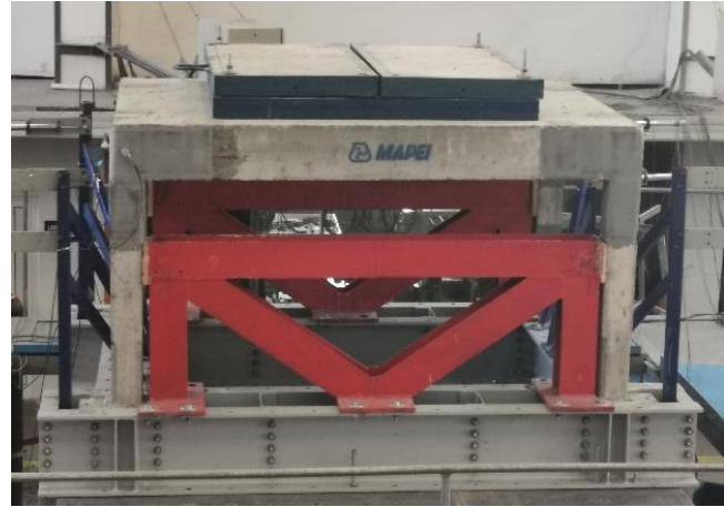
Fig. 2 – Designed experimental model to simulate short-column behavior
