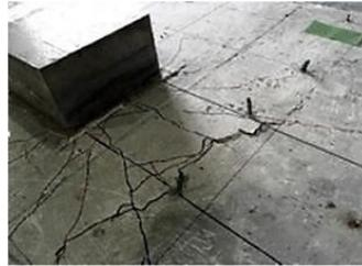
(e) Visible Failure Pattern (Experiment)[7]
