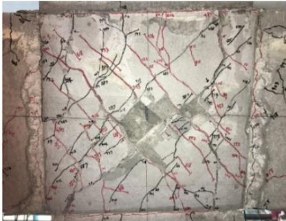
(2) J-21 specimen beam-column joints
