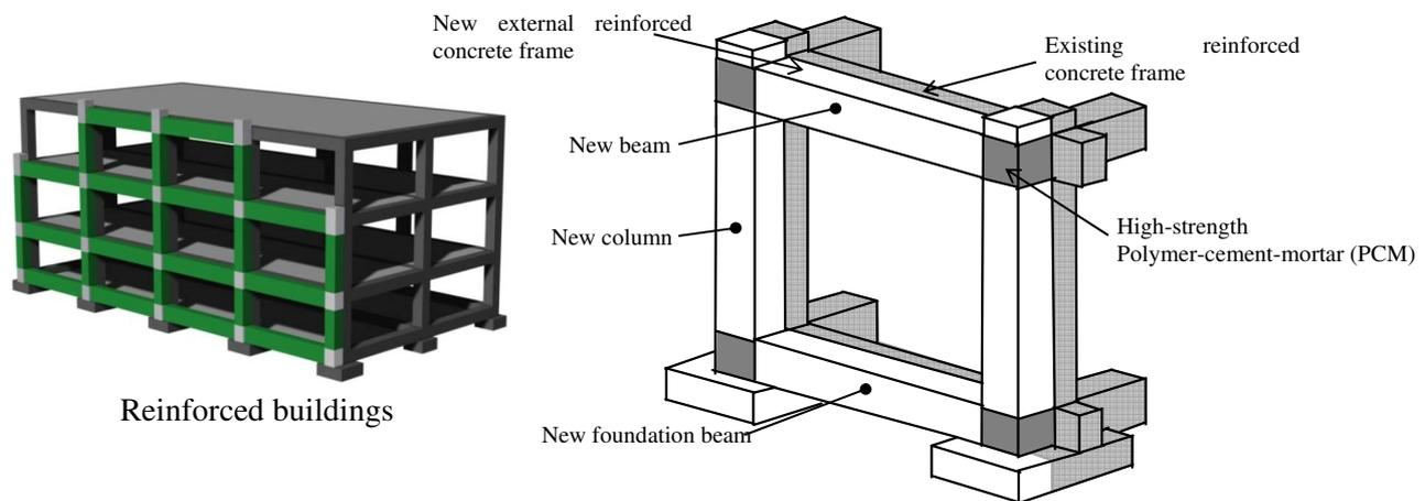
Fig. 1. Seismic retrofitting method using external frame
