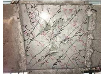
(3) J-22 specimen beam-column joints
