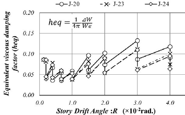
Fig. 7. Equivalent viscous damping factor
