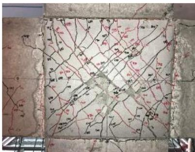
(4) J-23 specimen beam-column joints
