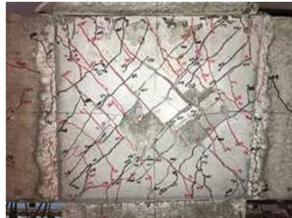
(1) J-20 specimen beam-column joints
