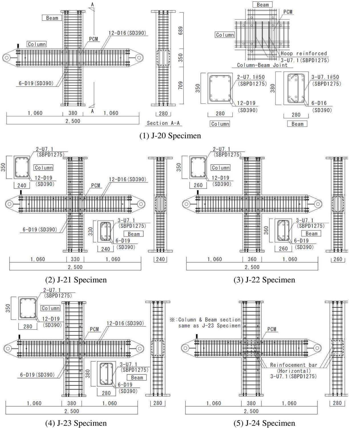
Fig. 2 . Shapes and the arrangement of reinforcing bars of specimens
