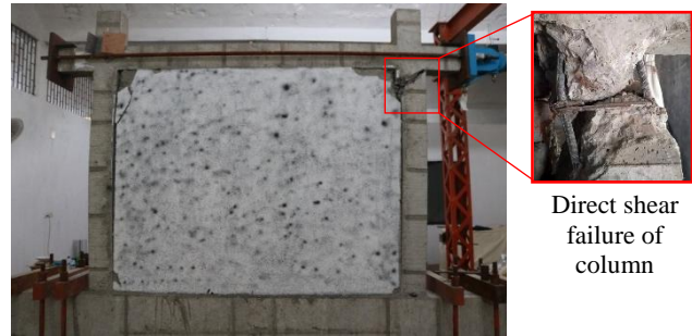
Fig. 10 – Final damage of Ferro-cement Laminated specimen (IM-FC)
