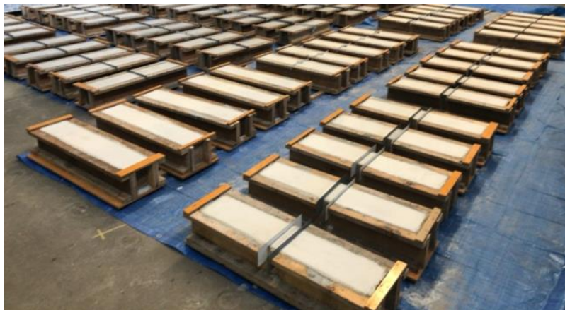
Pic. 2 – Conditions of curing (pre mold)
