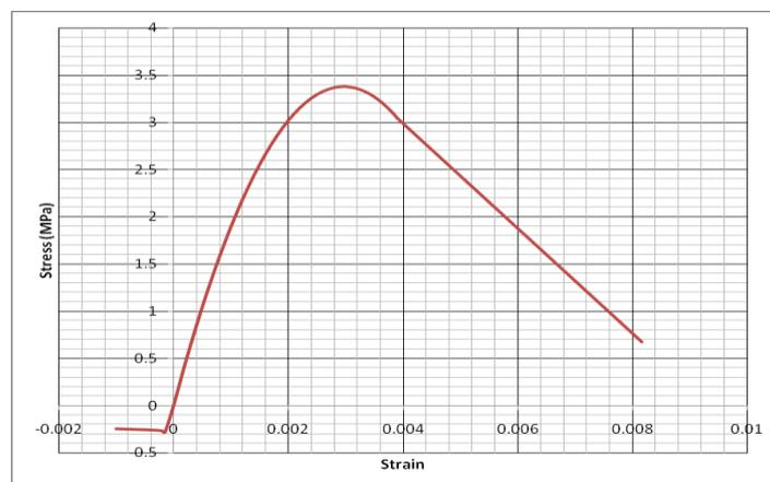
Fig. 4 Stress-strain curve for Masonry
