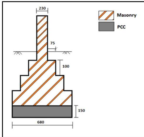
Fig.2 Existing foundation system
