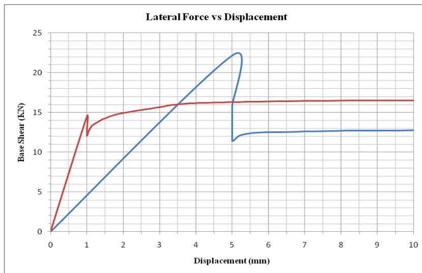
Fig. 8 Lateral Load vs Displacement graph for the foundations
