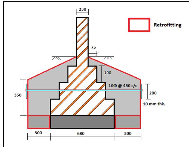
Fig.3 Retrofitted foundation system
